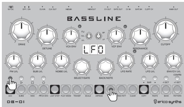
Push and hold the SHIFT button and push the LFO button to access the LFO settings! Rotate the SELECT/GATE encoder to select the function - LFO shape (SHP), synchronized/free running (SYC) LFO or LFO reset on each active step. Rotate the BACK/NOTE encoder to make a selection. The step buttons will give visual feedback of the LFO in action.
