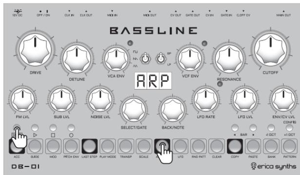
The DB-01 has a built-in arpeggiator. It can work in two ways – it can create simple arpeggios or insert arpeggios into the sequence.
