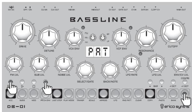
Once you are happy with a sequence that you have designed, you can **SAVE** it in one of the 16 pattern destinations in a selected bank. Push and hold the **SHIFT** button and push the **PATTERN** button. The step buttons, representing the pattern slots, will appear 70% dimmed, but slots with already saved patterns will be fully lit.
