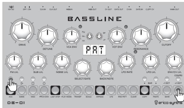
If you wish to recall previously saved patterns, push and hold the **SHIFT** button and push the **PATTERN** button. The step buttons, representing the pattern slots, will appear 70% dimmed, but slots with already saved patterns will be fully lit. Now push the regarding step button for the pattern you want to load and pattern will be loaded. If the sequencer is running it will complete the pattern that is playing, and only then load the new one.
