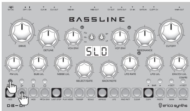
Push and hold the SHIFT button and push the SLIDE button! The sequencer will advance to the slide entry mode. You will see 70% dimmed step buttons showing which steps are active in the sequence. Push the step buttons for steps that you wish to slide, and step button LEDs will go on full brightness. With the slide activated the pitch of the activated, step will slide to the one for the next active step. To return to the step enter menu, push the BACK/NOTE encoder.
