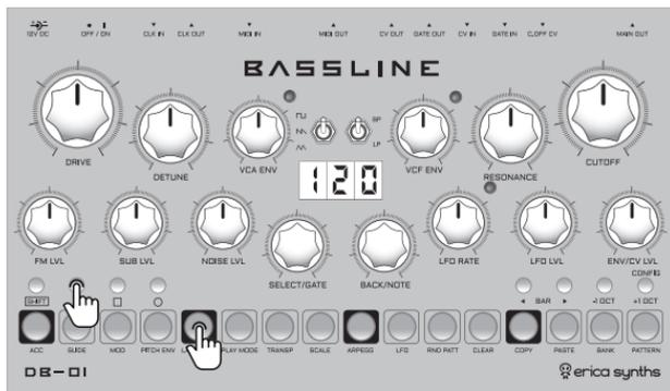
Connect the main output of the Bassline to the mixer. Push the BACK/NOTE encoder and rotate it while pushed to change the BPM rapidly by 10 (100-110-120-130, etc.)
