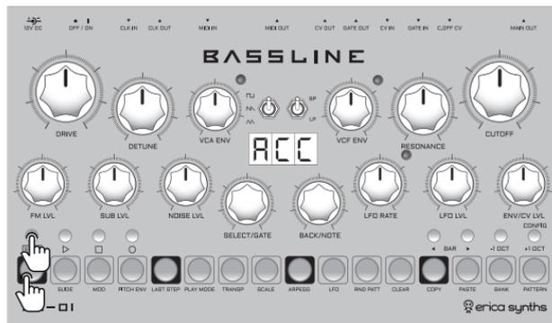
Push and hold the SHIFT button and push the ACC (accent) button! The sequencer will advance to the accent enter mode. You will see 70% dimmed step buttons showing what steps are active in the sequence. Push the step buttons for the steps that you wish to accent, and step button LEDs will go on full brightness. The accent will open the VCA and VCF slightly. To return to the step enter menu, push the BACK/NOTE encoder.
