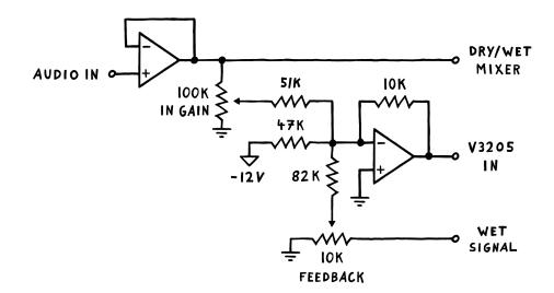
Using an 82k input resistor here will give us a feedback gain of about 1. Which would result in an infinite number of repeats. The circuit basically goes into self-oscillation. To be able to dial this back, we'll put a 10k potentiometer as a variable voltage divider between the wet output and the 82k resistor.
