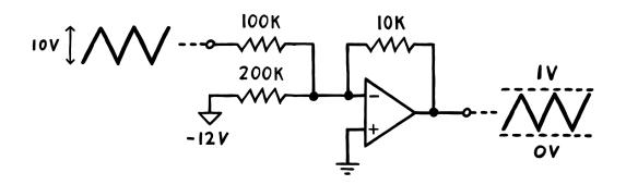
Since I plan to use audio from a eurorack synthesizer as our input, I assume that input to be a 10 V peak to peak signal that swings across the 0 V line. In that case, these resistor values will give us an approximately 1 V peak to peak result that is swinging just above the 0 V line.
