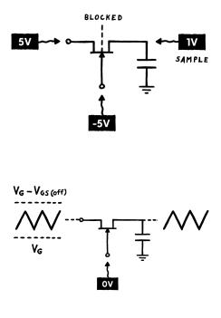
Next, we pull the gate voltage way below the source, disabling the JFET. This cuts the connection between signal and capacitor, which means that the charge is now trapped inside the cap. **This trapped charge is our sample**.
