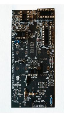
**Next, insert the first DIP socket,** hold it in place and solder one of the pins. Continue with the **next DIP socket.** Make sure the DIP sockets **are oriented correctly** – the notch on the socket should match the notch on the PCB's silkscreen. Now, turn the PCB around and solder all remaining pins of the DIP sockets.
