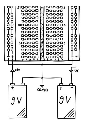
By connecting the batteries like this, the positive terminal of the left battery becomes your +9 V, while the negative terminal of the right is now your –9 V, and the other two combine to become your new ground.<sup>7</sup> Please make sure you disconnect the batteries from your breadboard when you make changes to the circuit! Otherwise you run the risk of damaging components.
