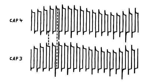
If we were to combine the two, we should be able to cancel out the clock oscillation, since the signal wouldn't jump between full and deficit state anymore. To test this, we'll simply set up another MOSFET buffer for cap 3 and then mix its output with the previous buffer using a simple passive mixer made of two 10k resistors.
