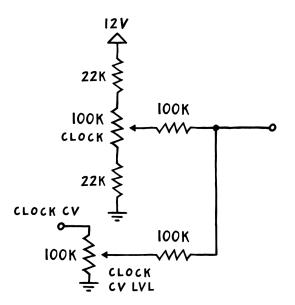
Okay, but what if there is no external signal plugged in at all? In that case, we would blast the 4046's CV input with 10 V – which it is not able to handle. To fix this, we simply add another variable voltage divider before the external CV input. This solves two problems at once. First, it provides a path to ground even if there's no external signal plugged in. And second, it allows us to change the intensity with which the CV affects the delay time.
