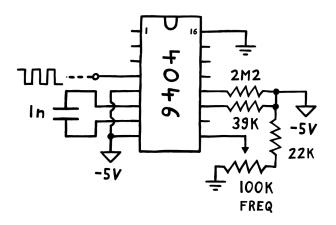
To use the VCO inside the chip, we first need to supply it with power. Since we want our clock to oscillate between 0 and -5 V, we'll give it 0 V as a high and -5 V as a low supply voltage. Next, we'll set the oscillator's frequency range. If we combine a 39k resistor to the negative supply at pin 11 with a 1 nF capacitor between pins 6 and 7, the VCO can produce clocks between 0 Hz and around 27 kHz.
