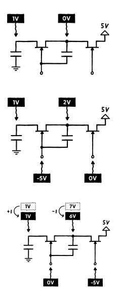
It works like this. We first add another JFET, which we connect to capacitor two on the left and a 5 V voltage source on the right. Then, we connect the other side of capacitor two to the gate of the first JFET (instead of connecting it to ground).
