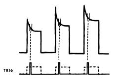
This shifts the trigger pulse to the right ever so slightly, allowing us to dodge the worst part of the clock spike. Okay, but our sampling window still contains a sizeable chunk of that spike. Wouldn't this show up in the output? It would if charging and discharging the sampling capacitor was instantaneous. But depending on the size of that capacitor, charging and discharging it takes a considerable amount of time.
