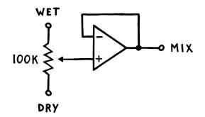
Then, we'll buffer the signal at the pot's wiper with a simple op amp buffer. **This way,** we've created an active mixer that allows us to apply different weights to both inputs simultaneously by turning a knob. Because we now draw current from our input in two separate places, I'm going to also buffer it – just to make sure we don't load the signal down and potentially distort it.
