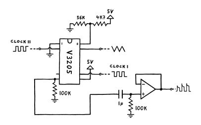
This means removing one output from the equation and killing the basic low-pass filter. However, we'll keep both the AC coupling and the buffer to ensure that we don't run into any headroom issues later on.
