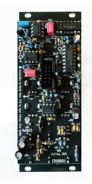
Now, **insert the ICs into their respective DIP sockets.** Mind the orientation of the ICs – match the notch on each IC with the one on its socket.
