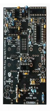
Once you are done with soldering the first batch of resistors, your PCB should look like this:
