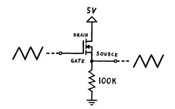
The core mechanism is very much comparable to a regular BJT emitter follower. The signal we apply to the MOSFET's gate is reproduced above the source resistor due to negative feedback. There are two important differences, though. First, a MOSFET's gate terminal is isolated from the rest of the device – meaning that it doesn't draw constant current from the signal we're trying to replicate. And second, a MOSFET's activation threshold can be much higher than that of a standard BJT.
