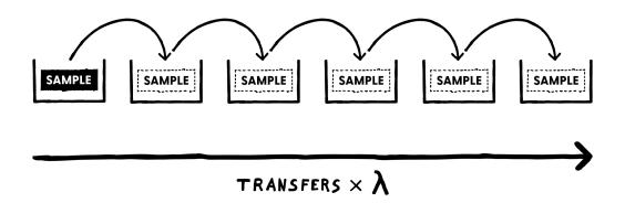
Since each transfer from one container to the next takes a small amount of time – one clock wavecycle, to be precise – the samples will reach the end of the chain with a time delay relative to the input. That time delay depends on the number of transfers and the frequency of the clock. If we then reconstruct the waveform from those delayed samples, we should get an output wave that's been shifted forwards on the x-axis (or in time).
