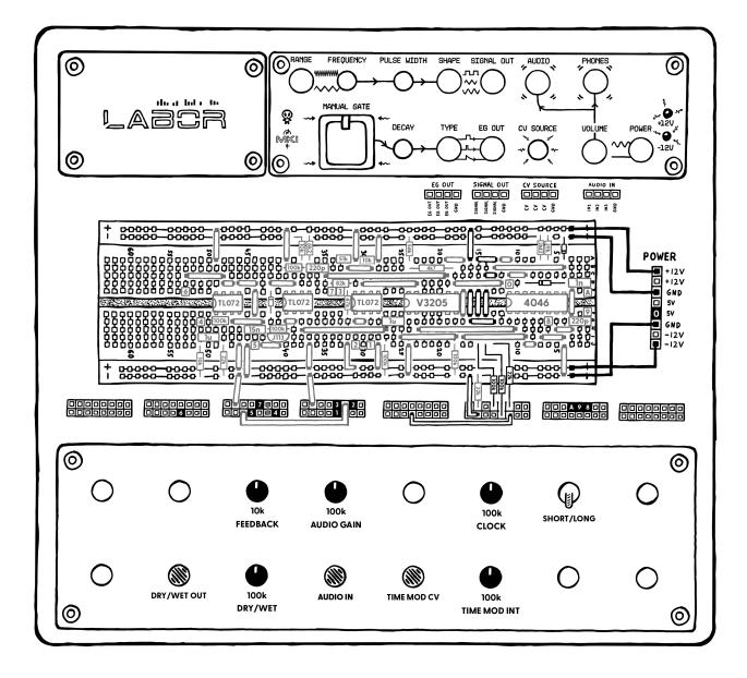
To test this, first try sweeping the delay time knob's range without any external CV applied. The range should stay roughly the same. Next, connect LABOR's oscillator to the clock CV input (while using something else for the audio input, of course). You should now be able to dial in different amounts of modulation going from subtle to extreme. Great!
