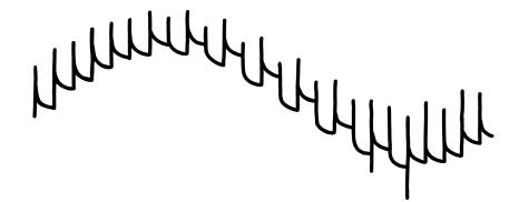
And second, the samples themselves also contain a clock spike, because the charge deficit transfer is not instantaneous. So what we're seeing here is one capacitor discharging into the previous one – until the deficit is fully transferred. To try and deal with this, BBD circuits usually apply an aggressive low pass filter to the output signal. To see how that would improve things, we can add a 10 nF capacitor to ground after our two resistors, creating a basic low pass filter.
