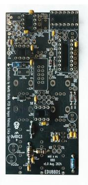
Then proceed with the **ceramic capacitors.** In order to avoid mistakes, first sort the capacitors by their values. Then place the PCB in your PCB holder or on spacers, insert the capacitors and solder them like you did with the resistors & diodes before. Now your PCB should look like this:
