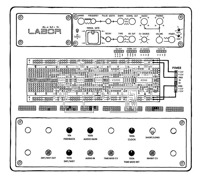
If you now apply a gate sequence to the new **inhibit cv** input, you should be able to create a fun rhythmic stuttering effect. Great! And with this, our bucket brigade delay is complete. Once you're done experimenting, dig out the panel and PCB from the kit, heat up your soldering iron and get to building. You can find more information on how to populate the board & how to solder in the enclosed appendix.
