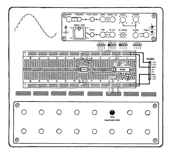
Okay. To start off, we're feeding LABOR's sine wave oscillator into our scaling and biasing sub-circuit (connection path 1), before routing it to a J113 JFET followed by a 15 nF capacitor. Then, we connect the clock generator, which receives its -5 V supply from LABOR's variable voltage source (connection path 0), to the JFET's gate. If you look at the output using an oscilloscope, you can see that the capacitor voltage looks like a sine wave – but with strange jagged edges. What's up with that?
