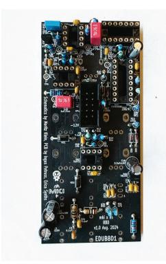
Then complete the component side of the BBD PCB by soldering the **PSU socket.** Make sure the orientation of the socket is as shown in the picture below – the arrow pointing to the first pin is aligned with a notch on the silkscreen. The key on the socket will be facing inwards towards the PCB. Now your PCB should look like this:
