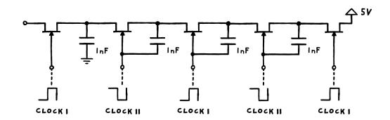
Then during the sampling phase (when clock one is high and clock two is low) JFET two will be closed, isolating the sampling stage and allowing it to operate just as we discussed earlier. And when the clocks flip, JFET one will be closed, kicking off the deficit transfer process.
