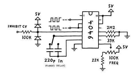
To protect the pin from voltages below 0 or above 5 V, we can repurpose the diode-based limiting approach that we just came up with.
