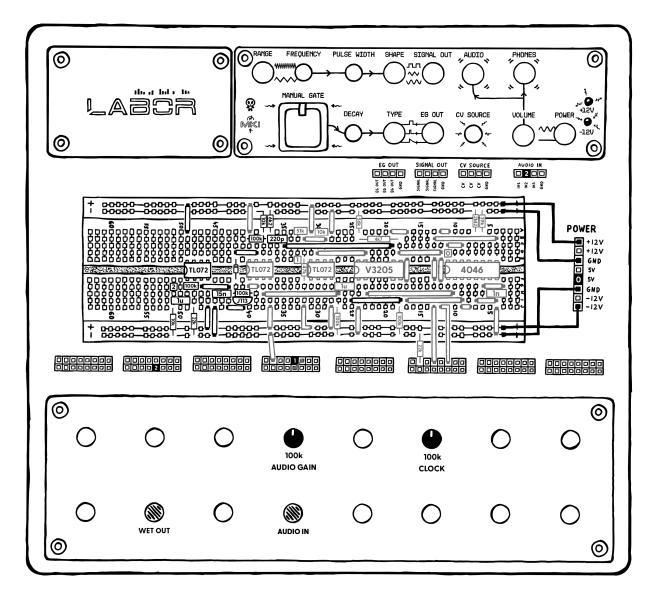
To see how all this works in practice, I recommend that you first compare the gate-totrigger converter's output to the clock signal on your oscilloscope. You should be able to see a clear gap between the clock's rising edge and the generated trigger. If you then swap the clock signal for the BBD chip's output, the trigger should be dodging the worst part of the spike as expected.
