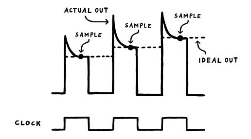
That voltage is the sample we took at the BBD's input. And we get that voltage in our actual output between the initial spike and the mid-clock cycle drop. So if we were to grab a small sample somewhere in that area and then hold that value until we grab the next one, we should be able to extract our ideal signal from the noisy BBD output. To try and implement this idea, we'll first need to undo our mixing and filtering approach.
