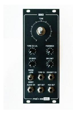
The LONG/SHORT switch requires special attention. Insert the switch in the relevant place on the PCB, place the front panel, fix it with few nuts on the potentiometer and jack sockets, then fix the switch with its nut (do not overtighten it) and then solder the switch.
