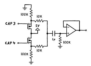
Since the reconstructed wave will have a significant DC offset, we'll then AC couple it using a 1 uF capacitor and a 100k resistor to ground. Finally, we'll add an op amp set up as a non-inverting buffer for a low output impedance.
