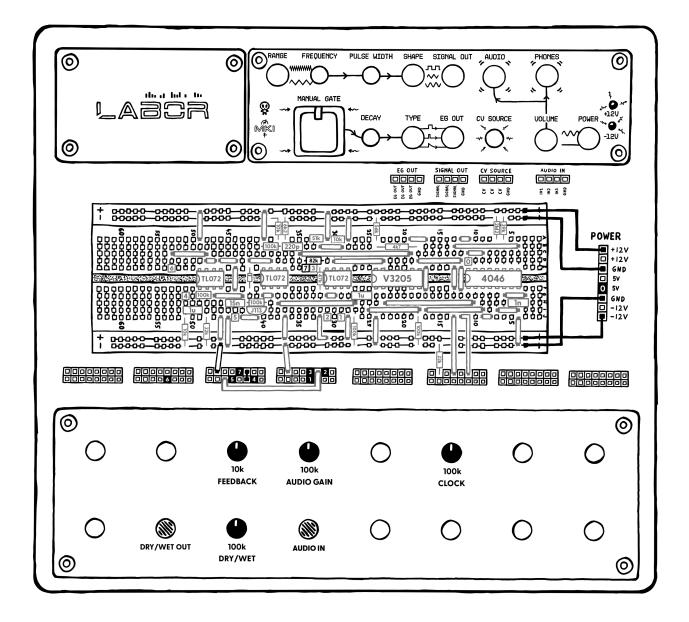
Using the new **feedback** potentiometer, you should be able to vary the number of repeats from just 1 to so many that the chip goes into wild self oscillation mode. Cool!
