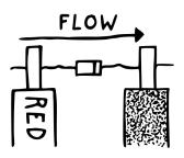
In some cases, it doesn't matter which probe you connect to which component leg or point in your circuit. This is true for testing resistors, non-polarized capacitors (foil/film, ceramic, teflon, glass etc.), continuity<sup>15</sup> or AC voltage.
