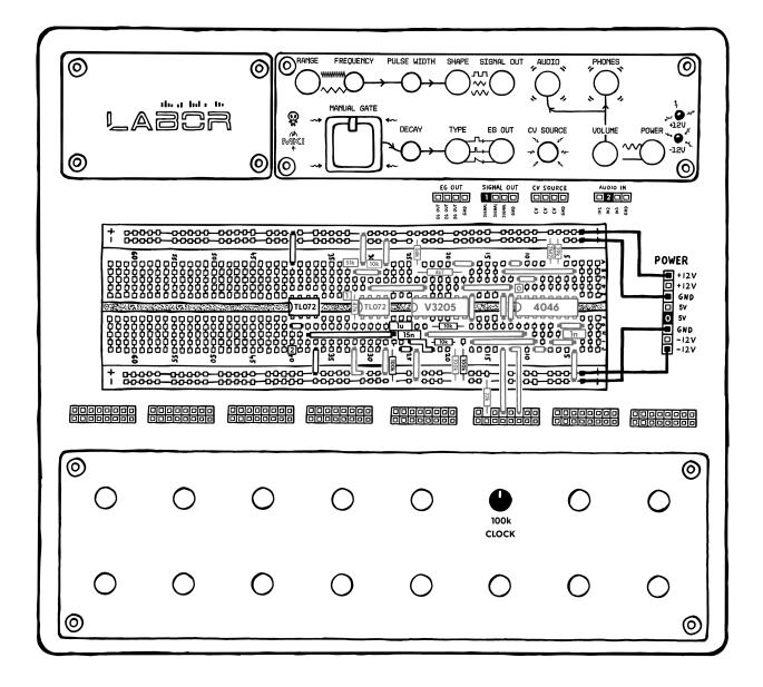
If you check out the output on your oscilloscope, the waveform should look and sound a little cleaner. It's not exactly *good*, but we'll get back to this later. **Because at the moment, our circuit is still pretty useless as a delay, since three transfers at a clock frequency of 10 kHz gives us an effective delay time of just 300 microseconds**. So if you overlay the input and the delayed output on your oscilloscope, you'll see just a very small shift on the x-axis.<sup>6</sup>
