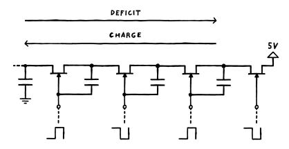
Note that to automate this circuit's operation, we'll need a second clock signal that is the exact inverse of our existing clock to drive every other JFET. Also note that each cap is only carrying information on every other clock pulse – it is either full (which means it's not carrying information) or at a charge deficit (which means that it is carrying information).
