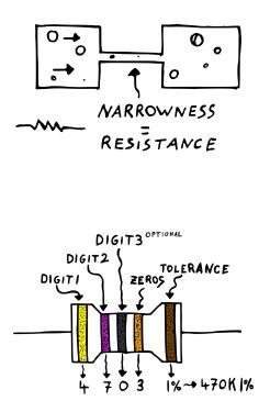
**Resistors have two distinctive properties: linearity and symmetry**. Linearity, in this context, means that for a doubling in voltage, the current flowing will double as well. Symmetry means that the direction of flow doesn't matter – resistors work the same either way.
