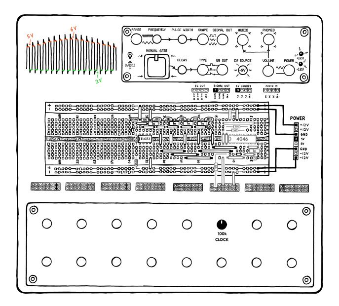
To try this, we'll add 3 BBD stages to our existing circuit. For the input, we'll use the same scaled and biased sine wave from before. Please note that some of the components used in this layout are not included in your kit. If you don't have these extra components in your stash, build the alternate layout below that uses kit components exclusively.
