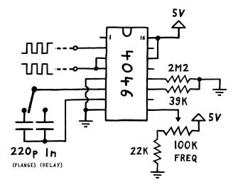
A 220 pF replacement gives us a frequency range of around 4 kHz to 112 kHz. Which should result in delay times ranging from around 1s to just 35 ms. And because I'd like to jump between delay and flanger mode on the fly, I'll set up both capacitor options behind a simple SPDT switch.
