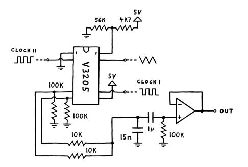
Then, we'll send clock 1 into pin 6, clock 2 into pin 2, and our scaled and biased input into pin 7. Finally, we'll drive our output reconstruction circuit from pins 3 and 4.
