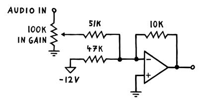
Next, we'll have to reduce the input resistance to increase the output's gain and make use of the available headroom. Because we might want to send in signals that are lower in volume than the eurorack-standard 10 V peak-to-peak, we'll drop that resistance down to 51k – and then insert a 100k variable voltage divider between it and the signal. This way, we can dial in the appropriate input gain for a wide range of signals – instead of fixing it to a value that only works for a specific type.
