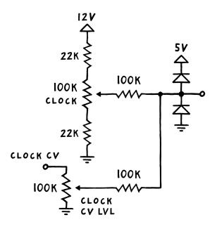
If we simply add in two diodes after our mixer – one pointing up to the 5 V rail and one pointing up from ground – then the voltage at the chip's input can never go significantly above 5 or below 0 V. That's because if it tries to, the diodes conduct and thereby neutralize the unwanted in- or decrease.
