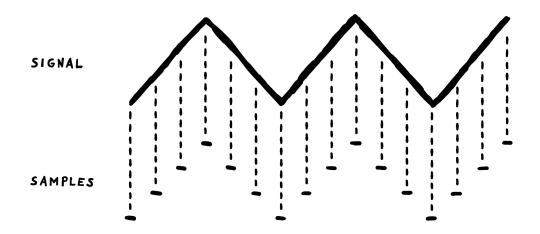
To extract a sample from this means that we probe the signal at any point and store whatever value we read. If we do this continuously and in regular intervals, we get a series of samples that resembles the input. But unlike a swinging voltage, those samples are discrete and can be easily held in a capacitor, allowing us to control when and how they move through the rest of our circuit.
