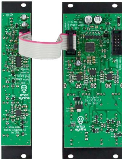
Select Logic or CV output for each envelope stage! Logic output means, the module outputs +5V gate signal when the relevant stage is active.
