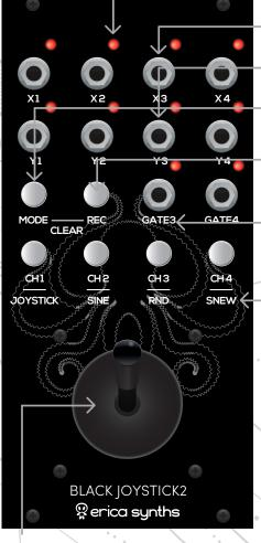
In order to access configuration, power a modular case off, push and hold the MODE button, and power the case on. Now, you can push CH1 button to engage the joystick position save and CH2 button to engage recall of last active channel. If the option is engaged, the relevant channel button will be lit.
