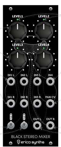
Small LEDs indicate signal level in each mixer channel. LED is full on if the signal level is 6Vptp
