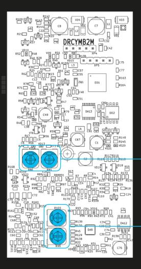
There are 4 trimpots on the back of the module to adjust presets of your module.
