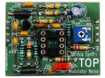
For Zener diode-based noise module solder all diodes, resistors (they are placed vertically; you may want to replace them with 0805 smt resistors) and DIP socket!
