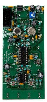
Turn the PCB around and solder potentiometers, jacks and mode switch!
