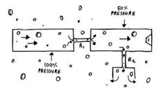
A voltage divider is really just two resistors set up like this: input on the left, output on the right. If R1 and R2 are of the same value, the output voltage will be half of what the input voltage is. How does it work?
