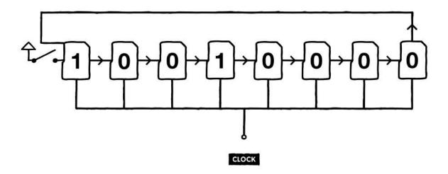
Add a few more logic 1s, and you've got a full drum pattern rotating through the chip. Okay, but how do we use this to trigger a drum sound? Easy: we just watch the very first cell. It goes high whenever a 1 swings by, essentially playing back what we tapped in. That's our trigger signal.
