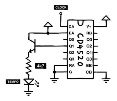
Now, when we feed it our 16th-note clock, the chip begins counting pulses in binary. Q0 toggles at half the input speed, giving us eighth notes. Q1 is half again, giving us quarter notes – and so on. For now, we'll grab the quarter-note pulse from Q1, buffer it with an NPN transistor, and use that to drive our clock LED. Finally, we'll disable the second counter by pulling its clock input low, so it stays inactive.<sup>8</sup>
