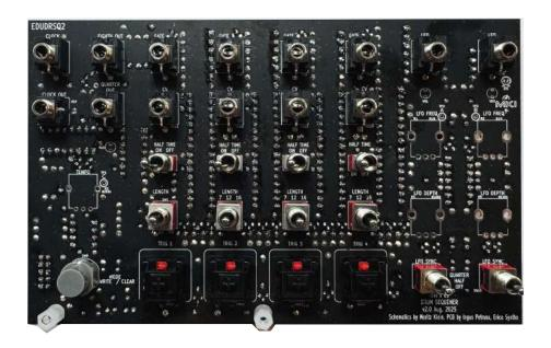
Insert **potentiometers**, but **don't solder** them yet! Also, install the **3mm LEDs** (make sure, the notch on the silkscreen is aligned with the one on the LED), but do not solder them!
