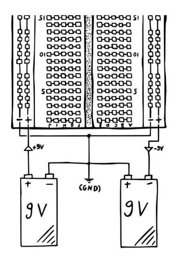
By connecting the batteries like this, the positive terminal of the left battery becomes your +9 V, while the negative terminal of the right is now your -9 V, and the other two combine to become your new ground.<sup>17</sup> **Please make sure you disconnect the batteries from your breadboard when you make changes to the circuit!** Otherwise you run the risk of damaging components.
