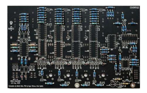
Next, insert the first **DIP socket**, hold it in place and solder one of the pins. Continue with other DIP sockets. Make sure **the DIP sockets are oriented correctly** – the notch on the socket should match the notch on the PCB's silkscreen. Now, turn the PCB around and solder all remaining pins of the DIP sockets. Compare your socket placement with the one on the picture below.
