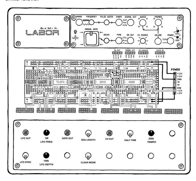
Once you've set this up, try patch the new CV output to the accent input of your drum module and hear how it sounds. (You can use the 16th note clock as a trigger signal.)
