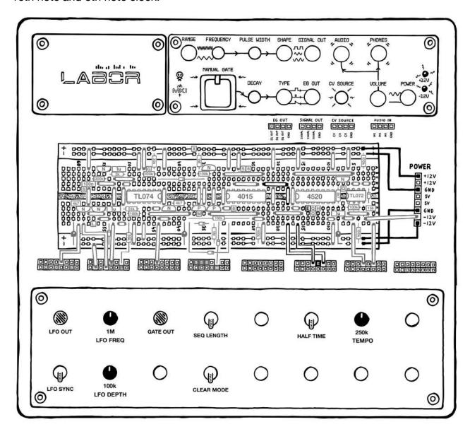
Switching to the 8th note clock should slow the playback speed down significantly. In the finished module, this will be very useful when you set one channel to half time mode, and another to the regular playback speed.
