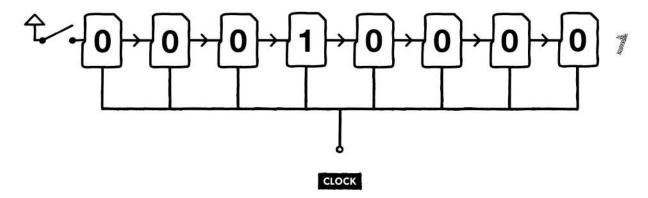
On each clock pulse, it shifts its contents one step to the right – while grabbing a new bit from the input. (A high voltage is interpreted as a logic 1, a low voltage as a logic 0.) Once a bit reaches the end of the chain, it drops off. But here's the trick: **if we connect the last cell back to the input, that bit circles around instead,** looping through the register indefinitely.
