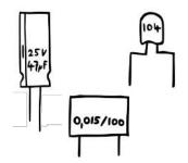
**A bunch of capacitors**. The specific values (which are printed onto their bodies) are
