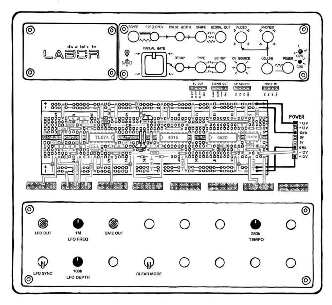
Try filling the entire register up with steps, then flip the clear mode switch and press the trigger button. You should be able to remove steps this way. Great! So now we have two voices (in theory), full control over each pattern, plus dynamic accents – all with just three buttons total. Not bad.
