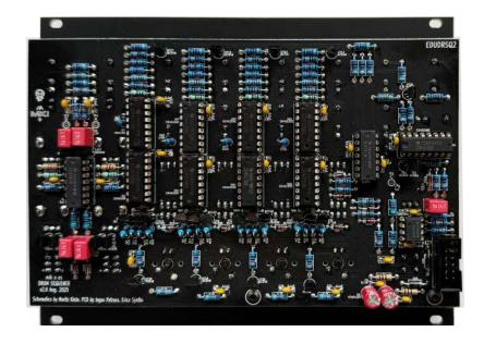
Congratulations! You have completed the assembly of the mki x es.edu Drum Sequencer module! Connect it to your eurorack power supply and switch it on. If there's no "magic smoke", it's a good sign that your build was successful. The module does not need calibration and, if your assembly is correct, it has to work straight away. Connect trigger outputs to some percussion modules and make a sequence!. **Enjoy!**
