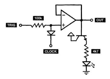
Speaking of power draw: to avoid overloading the op amp's output stage in the long run, we'll drive the LED through an NPN transistor.
