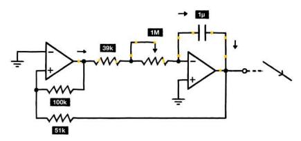
The integrator op amp is wired to neutralize any voltage change at its inverting input, so it counteracts by pulling current out of the other side of the capacitor. This results in a downward voltage ramp at its output. **Next, when the output has dropped far enough, the Schmitt trigger flips to its low state**. Now current flows the other way, causing the integrator's output to rise.
