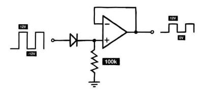
This lets positive voltages pass – while blocking anything negative. And to keep the output impedance low, we buffer the result with an op amp. Which we'll then hook up to the 4015's **CA** and **CB** clock inputs.<sup>4</sup>
