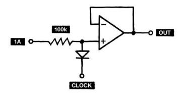
Here's how it works. Whenever the clock is high, the diode blocks, and whatever voltage is present at the trigger output gets buffered by the op amp unchanged. But when the clock is low and the trigger output is high, the diode conducts, pulling the voltage at the buffer's input low. As a result, the op amp's output drops as well – creating a clean rising edge on the next clock pulse.<sup>6</sup>
