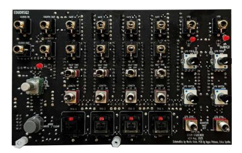
Fit the front panel, screw the nuts on the green potentiometer, jack sockets and switches and make sure that the potentiometer shafts are aligned with the holes in the panel – and that they're able to rotate freely. Now, go ahead and **solder the potentiometers and the LEDs** after fitting them in relevant holes on the front panel.
