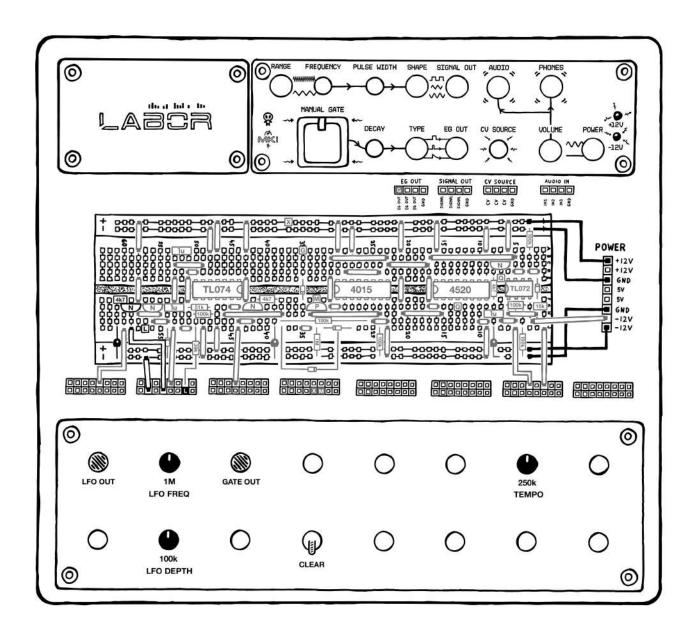
Try turning the depth knob as you apply the LFO's output to your drum module's accent input. You should be able to hear the maximum accent level drop. At the lowest setting, the drum hits all come out at the same low level intensity. Crank it up, and we're back to the full dynamic range.
