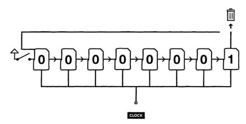
So if we could momentarily break the feedback loop by pressing a button – we'd be set. Implementing this isn't straightforward, though, because most push buttons are *normally open*: they only connect when pressed. **So if we'd put one into the feedback loop, the connection would be broken by default, and the sequence wouldn't loop unless we held the button down the entire time**. (Which is not very fun.) To work around this, we'll use a PNP transistor.
