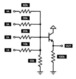
Here's how it works. We take four outputs from the shift register — let's say 1A through 4A — and run each through a resistor into the same point, like a simple passive mixer. But instead of using identical resistors, we'll pick values that roughly double from one to the next. This way, each output has double the weight of the one preceding it – just like bits in a binary number. This gives us 16 distinct voltage levels between 0 and 12 V, all evenly spaced.
