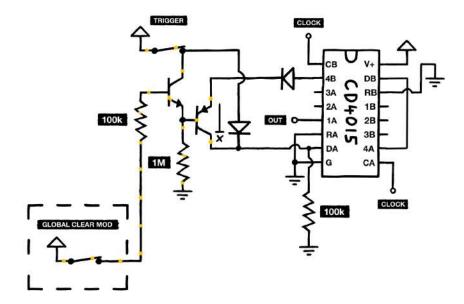
When both buttons are pressed, that NPN turns on, allowing current to flow. **This raises** the PNP's base voltage, which turns it off and breaks the feedback loop. But if either button is inactive, the NPN stays off and the loop continues.
