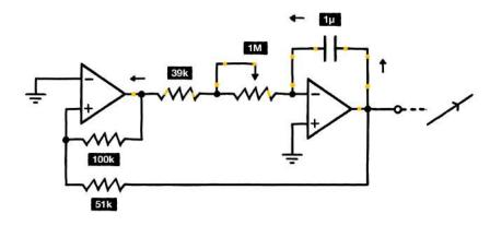
Eventually, that output climbs high enough to trigger another flip – and the cycle repeats. Unfortunately, there is one issue with this circuit. The output it produces swings between approximately 5 V and -5 V. This is a problem, because some drum voices will not produce any sound when given a negative accent voltage. To fix this, we'll need to lift the triangle above the 0 V line. How do we do that? Easy. All we need is a simple clamping circuit.
