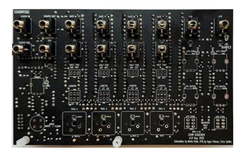
**Toggle switches** on the module require special attention. All components on the front panel are 10mm tall, except switches, therefore before soldering they must be tightened against front panel. Insert all switches, but **do not solder them, yet!**
