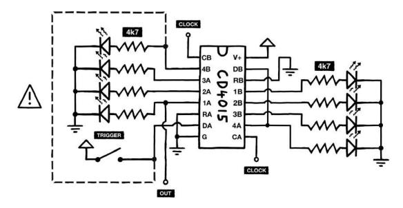
That's because both the output and the button are able to sink current – **meaning that if** either is high while the other is low, we create a short circuit. To avoid this, we'll set up two diodes – one after the button, and one at the **4B** output pin.
