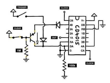
What we want now is to trigger that same behavior, but only when both a new, global clear mode button and the channel's trigger button are pressed together. To pull that off, we'll add an NPN transistor wired like this.
