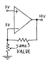
How about amplifying a signal though? To do that, we'll have to turn our buffer into a proper non-inverting amplifier. We can do that by replacing the straight connection between inverting input and output with a voltage divider, forcing the op amp to work harder. Here's how that works. Say we feed our non-inverting input a voltage of 5 V. Now, the output needs to push out 10 V in order to get the voltage at the inverting input up to 5 V. We call this setup a non-inverting
