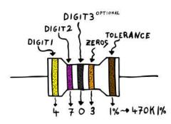
Resistors have two distinctive properties: linearity and symmetry. Linearity, in this context, means that for a doubling in voltage, the current flowing will double as well. Symmetry means that the direction of flow doesn't matter – resistors work the same either way.
