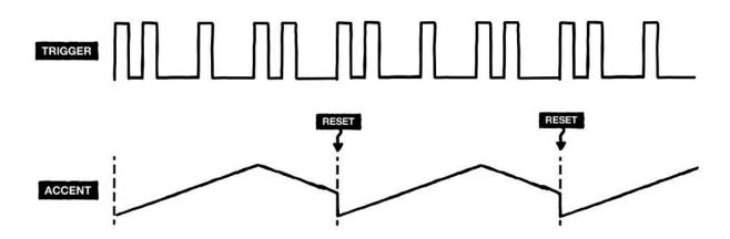
That would give us a perfectly repeating accent pattern – regardless of the triangle's base frequency. No drifting, no fine-tuning required. And while that might sound tricky to pull off, the actual solution is surprisingly simple.
