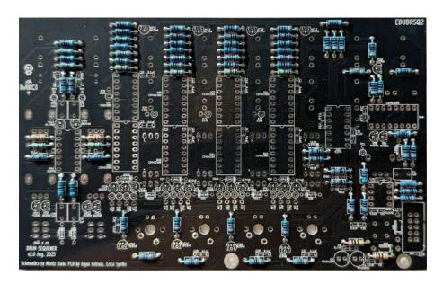
Now, proceed with **switching diodes** and the **power protection diodes**. Remember – **when inserting the diodes, orientation is critical!** A thick white stripe on the PCB indicates the cathode of a diode – match it with the stripe on the component. Solder all diodes.
