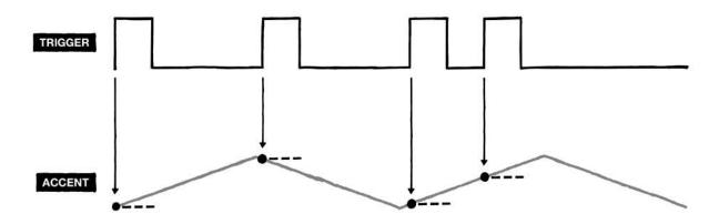
To generate a triangle wave, we'll set up a simple oscillator.
