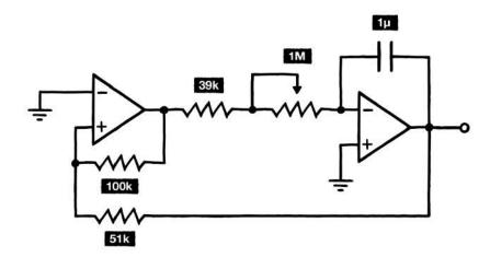
I've explained how this topology works in detail in our FM Drum manual, but here's a quick recap. The circuit combines two building blocks: a Schmitt trigger (left opamp) and an integrator (right op-amp), connected in a feedback loop. On power-up, the Schmitt trigger latches either into its low or high state – let's assume it starts high. This pushes current through the integrator's input resistance and into the capacitor.
