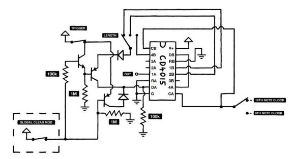
One side connects to the main 16th-note clock. The other taps into the 8th-note output from our clock divider.
