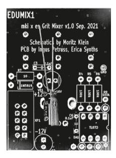
Then populate **film capacitors** and **2x5 PSU socket**. Make sure the orientation of the socket is as shown in the picture below – the arrow pointing to the first pin is aligned with a notch on the silkscreen. The key on the socket will be facing outwards the PCB. Now your PCB should look like this:
