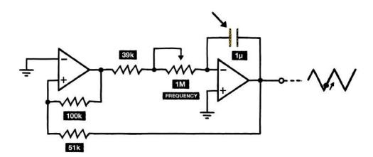
If we suddenly even it out, the oscillation should snap back to its starting point. Okay – but how do we do that? Easy: we just need to bridge the capacitor with a resistor and an NPN transistor.
