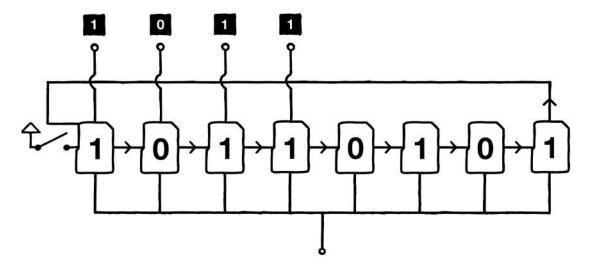
With four outputs, we get 16 distinct values. Now, here's the trick. We can convert each value into a corresponding analog voltage — and use that as our accent level. **Instead of just on/off, we'd then get stepped intensity: soft hits, loud hits, and 14 steps in between**. And the best part? We can do that conversion with just a couple of resistors and a buffer.
