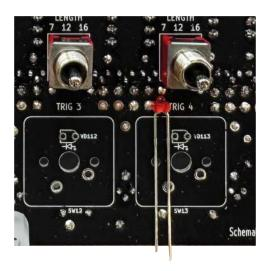
Now, adjust position of the cherry key, so it aligns with the silkscreen on the PCB and solder the second lead of the cherry key. Then proceed with other three cherry keys in the same manner. Also, populate and solder a pushbutton; make sure the notch on the pushbutton is aligned with the silkscreen. After completing this step, your PCB should look like this.
