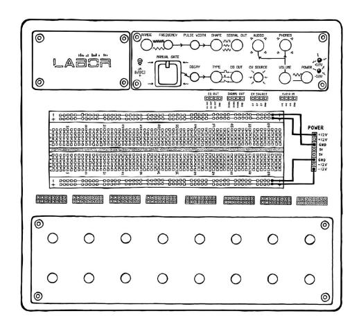
Before you get started, connect the slots labeled **GND** on the power header to both breadboard rails labeled – (minus). Next, connect one slot labeled +12 V to the top breadboard rail labeled + (plus), and one slot labeled -12 V to the bottom breadboard rail labeled + (plus).
