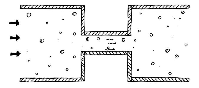
In that metaphor, resistance would be the width of a pipe. The wider it is, the more water can travel through it at once, and the easier it is to push a set amount from one end to the other. Current would then describe the flow, while voltage would describe the pressure pushing the water through the pipe. You can probably see how all three properties are interlinked: more voltage increases the current, while more resistance to that voltage in turn decreases the current.
