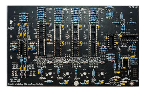
Next, insert and solder transistors. There are **PNP and NPN** transistors in the kit, therefore before soldering them, I highly recommend to **sort them.** Make sure you install them in correct places and pay attention on the orientation of the transistors – notch on the silk-screen has to match the flat part of the transistor.
