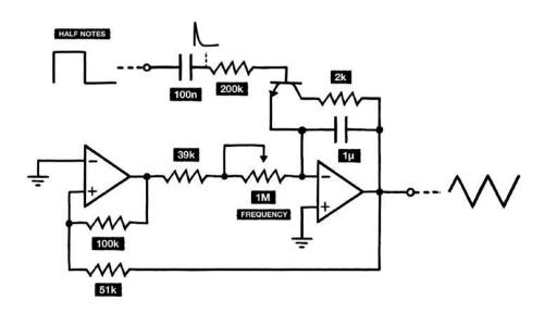
The cap only lets a quick burst of current through – right when the 4520's output first goes high – creating the short pulse we need. And we can even take this a step further by setting up a three-way switch so we can either let the LFO run freely, sync it to the full pattern length, or sync it to half the pattern length for even straighter accents.
