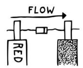
In some cases, it doesn't matter which probe you connect to which component leg or point in your circuit. This is true for testing resistors, non-polarized capacitors (foil/film, ceramic, teflon, glass etc.), continuity<sup>25</sup> or AC voltage.
