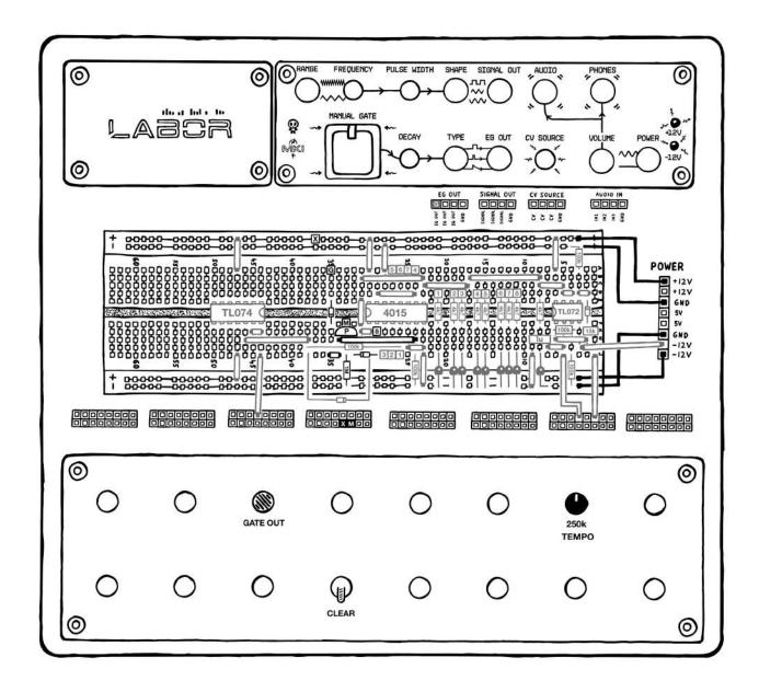
Since your kit does not contain a breadboard-friendly push button, we'll need to use a switch as a replacement. Let's see if it works: fill up the register with bits, then try removing some by briefly flipping the switch.<sup>7</sup>
