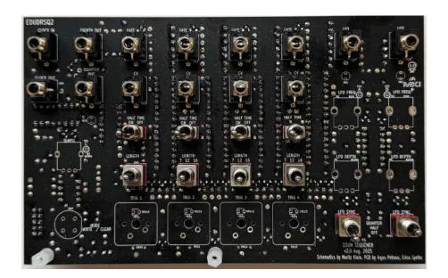
Install the front panel and fix it with few hexnuts on the jack sockets and two M3 screws for spacers. Then **tighten hexnuts** on switches so that switches are firmly **pushed against the front panel**; you may want to adjust alignment of the single pole switches as they tend to be bit loose in their places.
