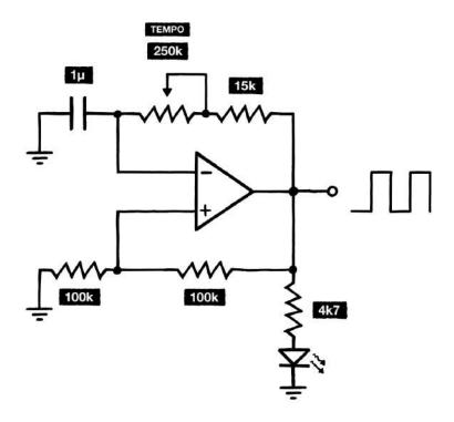
I've explained this exact clock oscillator in the manual for our DIY sequencer kit<sup>2</sup> in detail, but here's the basic gist. The op amp is wired in an intentionally unstable way, forcing it to charge and drain the capacitor on the left in an endless loop.
