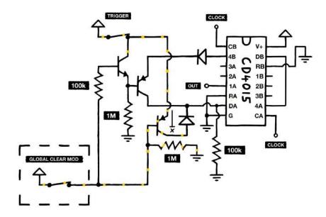
It works like this: when clear mode is off, the PNP conducts, and trigger presses behave normally. But when clear mode is on, the PNP shuts off — cutting the connection
