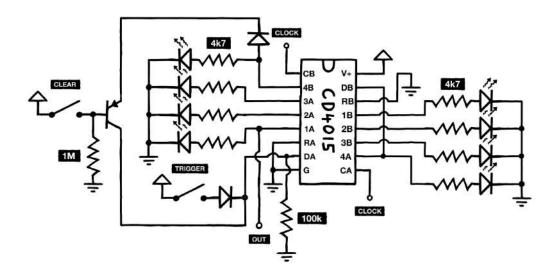
If we place it in the feedback loop like this, it conducts by default – unless its base gets pushed high by the button, in which case it blocks and breaks the loop.
