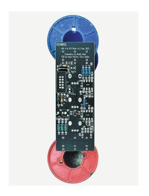
Place the Snare Drum PCB in a PCB holder for soldering or simply on top of some spacers (I use two empty solder wire coils here).
