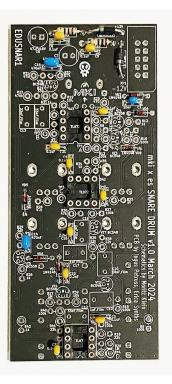
Next, insert the first DIP socket, hold it in place and solder one of the pins. Continue with the next DIP socket. Make sure the DIP sockets are oriented correctly – the notch on the socket should match the notch on the PCB's silkscreen. Now, turn the PCB around and solder all remaining pins of the DIP sockets. Then insert and solder the ceramic capacitors.
