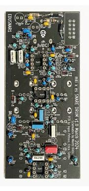
Now, proceed with other vertically placed resistors. If you are not sure about resistor value, use the multimeter to measure resistance of each resistor before soldering them. Once you have completed installing the resistors, your PCB should look like this:
