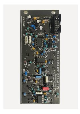
Now, insert the ICs into their respective DIP sockets. Mind the orientation of the ICs – match the notch on each IC with the one on its socket.
