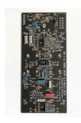
Then proceed with **the film capacitors.** Place the PCB in your PCB holder or on spacers, insert the capacitors and solder them like you did with the resistors & diodes before. Now your PCB should look like this:
