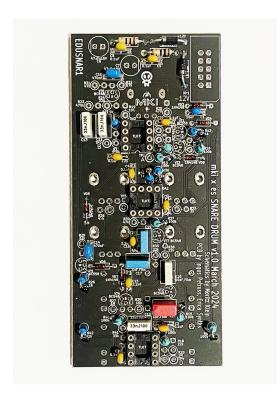
Because the Snare drum features quite few resistors, let's start with 100 k resistors (light blue on the photo to the left) and 1 k resistors (dark blue on the photo to the left). When those are installed, the PCB should look like this:
