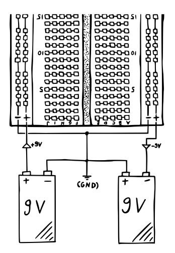
By connecting the batteries like this, the row on the left side labeled + becomes your positive rail, the row on the right side labeled + becomes your negative rail, and both rows labeled – become your ground rails.<sup>2</sup> Please make sure you disconnect the batteries from your breadboard when you make changes to the circuit! Otherwise you run the risk of damaging components.
