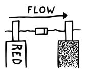
In some cases, it doesn't matter which probe you connect to which component leg or point in your circuit. This is true for testing resistors, non-polarized capacitors (foil/film, ceramic, teflon, glass etc.), continuity<sup>27</sup> or AC voltage.
