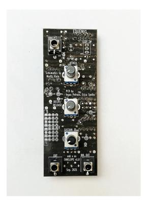
**Insert the potentiometers, but don't solder them yet!** Fit the front panel and make sure that the potentiometer shafts are aligned with the holes in the panel – and that they're able to rotate freely. Now, go ahead and solder the potentiometers.
