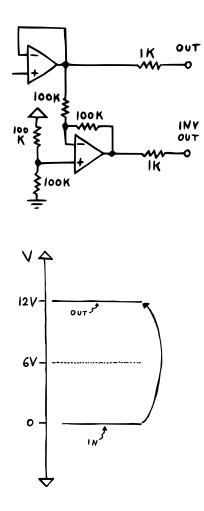
Turns out it's doable quite easily with another op amp, which we'll set up as an inverting buffer.<sup>15</sup> But instead of connecting the non-inverting input to ground – as you would normally do –, we give it a constant 6 V from a simple 50 % voltage divider.
