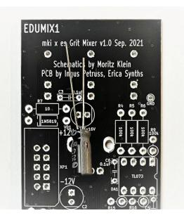
Next, insert & solder the electrolytic capacitors. Electrolytic capacitors are bipolar, and you need to mind their orientation. The positive lead of each electrolytic capacitor is longer, and there is a minus stripe on the side of the capacitor's body to indicate the negative lead. On our PCBs, the positive pad for the capacitor has a square shape, and the negative lead should go into the pad next to the notch on the silkscreen.
