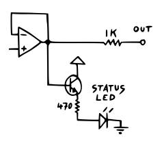
Here's how this works. Whenever our buffer sends out a non-zero voltage, a tiny current will flow into the transistor's base. This will cause that transistor to open up, resulting in a much bigger current flowing from the positive rail through the current limiting resistor and then our LED, lighting it up.<sup>14</sup>
