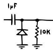
First a positive one, when the input transitions from low to high – and then a negative one when it drops from high to low. Now, since we're not interested in the negative spike, and it could cause our comparator to glitch out under certain circumstances, I've decided to eliminate it using another diode. Whenever the voltage at the comparator's input (i.e. after the 1  $\mu$ F capacitor) tries to go negative, the diode will open and thereby neutralize it.<sup>12</sup>
