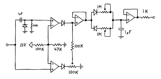
Here's how that would work. As you can see, I've basically just copied our comparator and pasted it down at the bottom. Both the new and the original one get the input signal, and they share the same reference voltage, but I've placed a high-pass filter before the top one. That high-pass would normally turn a square wave cycle into two short voltage spikes.
