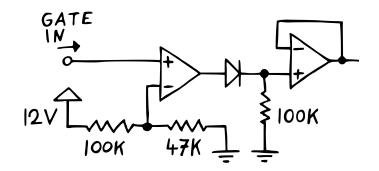
Here's what that does. Whenever the comparator is pushing out 12 V, the diode conducts and we also get about 12 V at the buffer's input. But once the voltage turns negative, the diode will block. Normally, the buffer's input would now be undefined (or "floating"). But since we have a 100k resistor to ground there, that input gets pulled down to 0 V instead.
