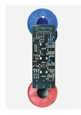
Place the Envelope PCB in a PCB holder for soldering or simply on top of some spacers (I use two empty solder wire coils here).
