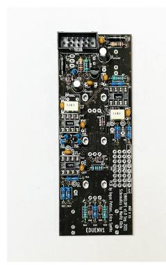
Next up: inserting & soldering the transistor. Make sure you align the transistor with the marked outline on the silkscreen – orientation is critically important here. Also, insert film capacitors and solder them.
