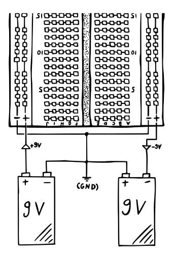
By connecting the batteries like this, the positive terminal of the left battery becomes your +9 V, while the negative terminal of the right is now your –9 V, and the other two combine to become your new ground.<sup>19</sup> **Please make sure you disconnect the batteries from your breadboard when you make changes to the circuit!** Otherwise you run the risk of damaging components.
