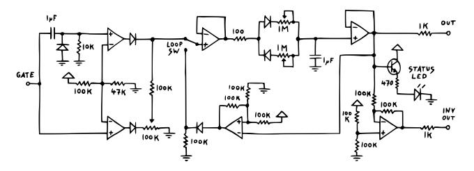
By circumventing the input comparators, the relation between our Schmitt trigger inverter's state and the envelope's output voltage becomes a lot simpler. Because now, there's no envelope setting that can prevent its output from peaking at a value below 8 V. The inverter will simply keep pushing out a high level voltage until we cross that threshold.
