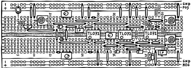
Try driving your VCF with the newly added inverted output. You should be able to verify that it now starts off open and then closes down as the envelope cycles through its phases.
