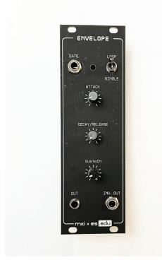
Now, insert the switch in the relevant place on the PCB, place the front panel, fix it with few nuts on the jack sockets and **solder the switch**.
