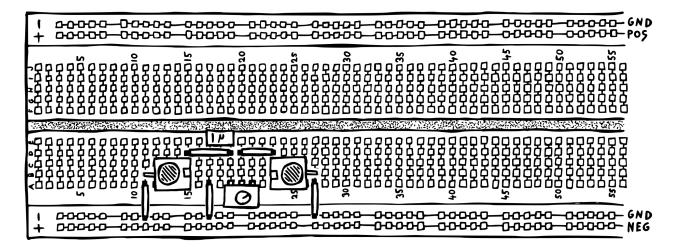
To properly test this circuit, you'll need a square wave LFO<sup>6</sup> and a module with a CV input like a VCF. Send in the LFO via the right-hand socket, while connecting the other one to your filter. By turning the potentiometer's knob, you should be able to dial in a more or less intense effect. Great! **The only problem with this is that the attack- and release phases are not adjustable independently**. Changing one will always also change the other.
