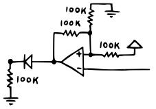
You just patch it in between output (on the right) and input (on the left) – and the envelope will re-trigger continuously. To make that happen, we're configuring yet another op amp as a Schmitt trigger inverter.<sup>17</sup> You can think of that like a watchdog which constantly monitors the envelope's output voltage. Whenever that output drops to 0 V, our watchdog will re-trigger the envelope and then sit back and wait until it's time to strike again.<sup>18</sup>
