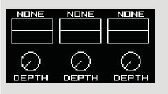
In the CV menu you can assign each of three CV inputs to different parameters of the Sample Drum, like tune, play mode, sample select, start, loop and end point, envelope attack, hold and decay, etc., as well as adjust modulation depth via attenuators.
