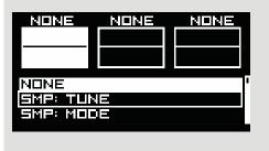
Rotate the encoder A/DATA to assign CV1 input to some of the parameters (TUNE is selected as the parameter in the example on the left) and push the encoder to confirm.
