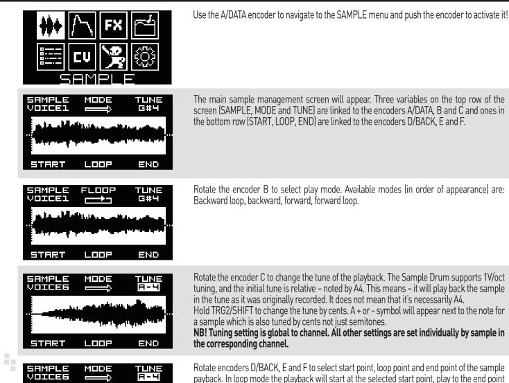
The main sample management screen will appear. Three variables on the top row of the screen (SAMPLE, MODE and TUNE) are linked to the encoders A/DATA, B and C and ones in the bottom row (START, LOOP, END) are linked to the encoders D/BACK, E and F.
