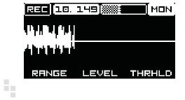
In RECORD mode you can record samples directly to the RAM of the module and afterwards save them to the SD card. Samples are saved as 16bit 48Khz way files. 12bits is the resolution of the ADC. Maximum record time is 30". To record the sample, patch the audio signal to CV3/REC (bottom row CV3) input.
