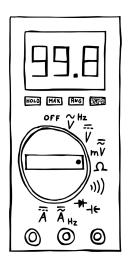
Multimeters come in different shapes and sizes, but the most common type is probably the hand-held, battery powered variant. It can measure a bunch of different things: voltage, current, resistance, continuity. Some have additional capabilities, allowing you to check capacitance, oscillation frequency or the forward voltage drop of a diode.
