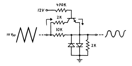
For this, we bridge the 10k resistor with a smaller resistor and another NPN transistor. Now when a voltage is applied to the NPN's base via a big resistor, it allows (forward) current to bypass the 10k resistor. This selectively reduces the amount of scaling we apply to the input, which causes one diode to open more quickly and widely, resulting in a much sharper cut-off at the positive tips of our triangle wave.
