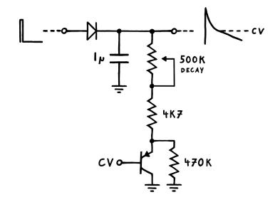
If we put a PNP transistor between the envelope's resistance and ground, the capacitor can only discharge to the voltage at the PNP's base – keeping the VCA open at that level. Since we still want the volume to decay further from here, if only slowly, we bridge the transistor with a big 470k resistor. This allows the cap to gradually discharge past the set CV level.<sup>14</sup>
