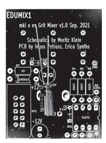
Insert & solder the electrolytic capacitors. Electrolytic capacitors are bipolar, and you need to mind their orientation. The positive lead of each electrolytic capacitor is longer, and there is a minus stripe on the side of the capacitor's body to indicate the negative lead. On our PCBs, the positive pad for the capacitor has a square shape, and the negative lead should go into the pad next to the notch on the silkscreen.
