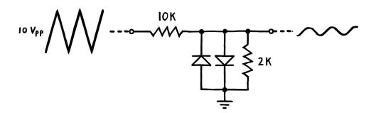
This will gently shave off the tips of the triangle, turning it into a rough sine wave. With the exact shape determined by the amount of scaling we apply: too little, and the tips become flat. Too much, and they become too pointy.
