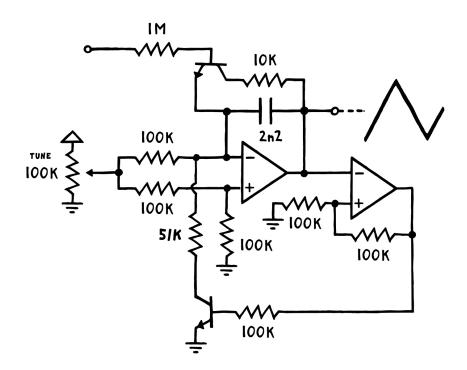
First, we'll use a significantly bigger capacitor in our integrator. This shifts the oscillator's frequency range downwards. This is desirable because it generally sounds more interesting if the modulator's frequency is lower than that of the carrier – at least in my opinion. And second, we'll push the schmitt trigger inverter's thresholds further apart so we get a stronger output to work with.
