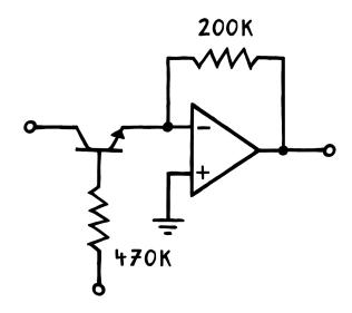
In essence, this design is just a regular inverting amplifier, but the input resistor has been replaced with an NPN transistor as a fake voltage controlled resistor. For this to work, the input signal needs to be extremely low in volume: just around 20 mV peak-to-peak. Then, the transistor will be locked into its saturation mode, where a large current flows into its base. This current's ultimate direction is then modulated by the tiny oscillation at the transistor's collector.
