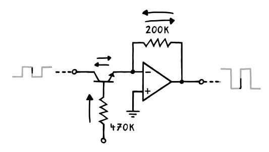
And since the emitter current depends on the base current, we can control the output signal's gain by changing the base voltage. And that's it: we've got a VCA!<sup>4</sup> Of course, since most input signals will be way too loud to keep the transistor in saturation, we'll also add a strong voltage divider at the VCA's input. Which can, conveniently, double as the scaling resistance for our waveshaping circuit, since it's essentially just a 2k resistance to ground.
