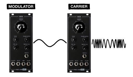
You take one VCO, which we'll call the carrier, and you modulate its frequency using the output of another VCO, which we'll call the modulator. This creates complex patterns in the output waveform of the carrier. Which, depending on the relation between the two oscillators' frequencies, can sound really harsh and aggressive. To implement this in our circuit, we'll simply clone our existing VCO to create a modulator – with two slight differences.
