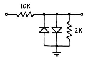
To understand how it works, let's assume that we apply our triangle to the resistor on the left. Then the other resistor going to ground will scale that triangle down: from around 10 V peak-to-peak to just 1.6 V peak-to-peak. Or rather, it would if it weren't for the diodes coming up from and going down to ground. Because as the triangle tries to push past the 400mV line in either direction, the respective diode will gradually open up and sink (or source) more and more current.
