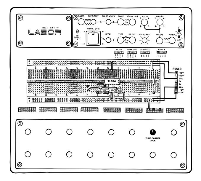
When you check the circuit's output on an oscilloscope (the Labor Scope add-on is great here), you should see that the integrator does produce a continuous triangle wave.<sup>2</sup> Using the CV potentiometer, which we've set up as a simple variable voltage divider between 12 V and ground, you should be able to adjust the oscillation frequency.
