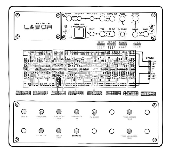
You should now be able to adjust the output's tail by applying different CV levels to the new DECAY CV input. Try it in the pulse wave mode as well, for simulating opening and closing hi-hats!
