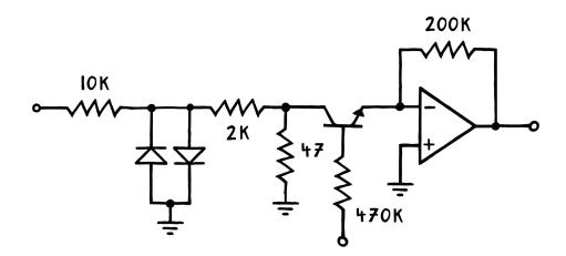
There is one small issue with this design. If you set this up on your breadboard, you'd notice that the output waveform has a positive DC offset that appears to be tied to the control voltage.<sup>5</sup> What's up with that?
