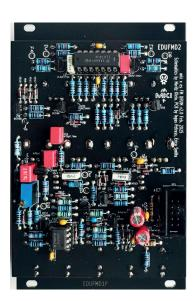
Now, insert the ICs into their respective DIP sockets. Mind the orientation of the ICs – match the notch on each IC with the one on its socket.
