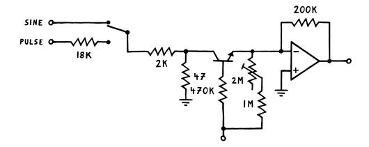
Because the pulse wave is much louder than the sine wave, we also need an additional 18k resistor to compensate. In combination with the VCA's voltage divider, this scales the pulse down to the proper input range for our VCA.
