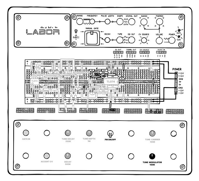
By flipping the FM ON/OFF switch, you should be able to turn on the circuit's FM mode. Try tuning carrier and modulator to different intervals and see what kinds of glassy/ metallic sounds you can create!
