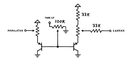
If we then apply a positive voltage to the transistors' bases, that voltage will be mirrored at the PNPs' emitters. And if the voltage below the potentiometers is raised above ground, their output voltages will increase proportionally. There's one caveat to this solution: since it's kind of a messy hack, we can't expect to get a v/oct response. Still, we can make it somewhat tuneable by adding a simple input attenuator.
