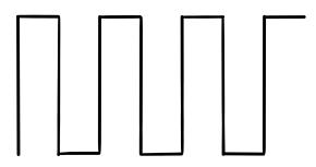
The **TP2** troubleshooting tips apply here as well, since the square signal is coming from the same oscillator. So we'd recommend using the signal at **TP2** for troubleshooting.
