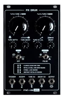
Finally fit the Tune potentiometer knobs and we are done!
