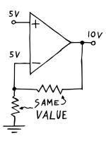
Before the op amp starts processing the voltages at its inputs, the output will be switched off. This means that **output and inverting input sit at 0 V at first**. So then, the op amp will subtract 0 from 5 and multiply the result by its gain. Finally, it will try and increase its output voltage to match the calculation's outcome.
