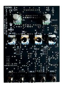
Next, **insert the top potentiometers and jack sockets,** then fit the panel to align components, you just installed, and solder them. Remove the front panel, insert other potentiometers, but don't solder them yet! Fit the front panel, screw the nuts on the top potentiometer and jack sockets and make sure that the potentiometer shafts are aligned with the holes in the panel – and that they're able to rotate freely. Now, go ahead and solder the potentiometers.
