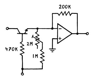
This way, we can dial in the ideal amount of compensation current for our specific transistor.
