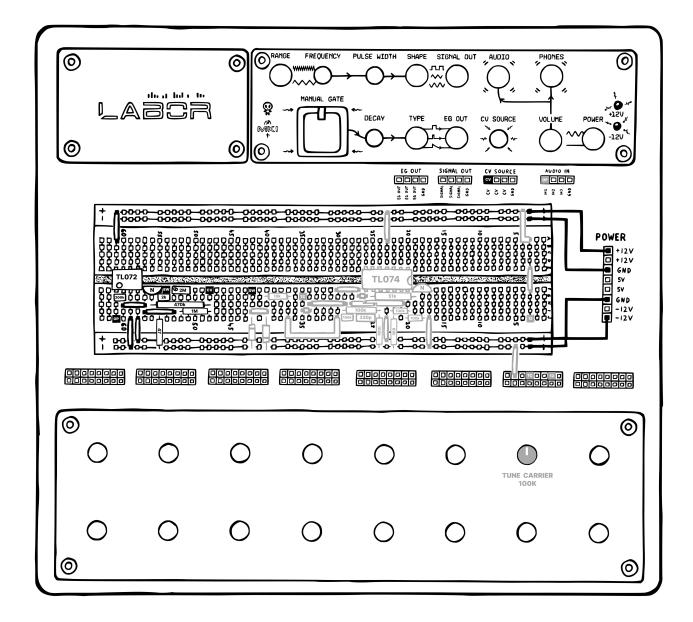
To center your sine wave, you'll need to view it on your oscilloscope and then fiddle with the trimmer until it's properly aligned with the 0 V line.<sup>6</sup>
