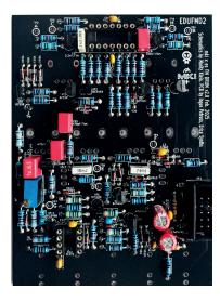
Then populate the trimpot and **2x5 PSU socket.** Make sure the orientation of the socket is as shown in the picture below – the arrow pointing to the first pin is aligned with a notch on the silkscreen. The key on the socket will be facing outwards the PCB. Now your PCB should look like this:
