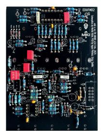
Then proceed with the ceramic capacitors. Start with soldering 0,1uF capacitors - place the PCB in your PCB holder or on spacers, insert the capacitors and solder them like you did with the resistors & diodes before
