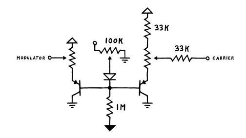
It works like this. The resistor ensures that a small current flows through the diode at all times. And when a current flows through a diode, there will be a diode drop across it. So for 0 V external CV, we'll get around -500 mV at the PNPs' bases. Which should then give us about 0 V at their emitters.<sup>15</sup>
