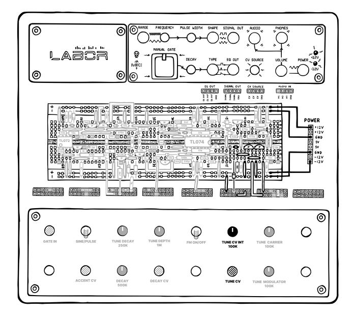
Try sending a CV sequence into the new TUNE CV input. By playing with the individual steps' CV values in combination with the TUNE CV INT potentiometer, you should be able to dial in some basic melodies. Great! And with this, our FM Drum is complete. Once you're done experimenting, dig out the panel and PCB from the kit, heat up your soldering iron and get to building. You can find more information on how to populate the board & how to solder in the enclosed appendix.
