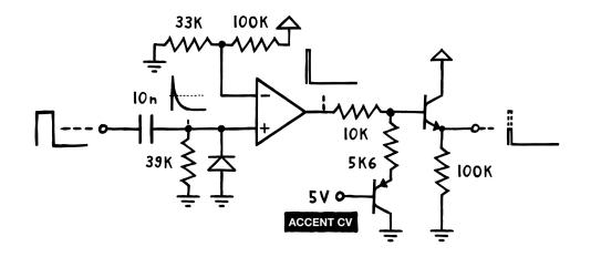
The Hi-Hat module's manual has an in-depth explanation, but here's the basic gist. The circuit uses a high pass with an added diode coming up from ground to turn an incoming gate into one quick, positive spike. Then, that spike is converted into a proper trigger (a quick pulse jumping from low to high and back) using a comparator. Finally, that trigger is sent into an accenting circuit which allows us to limit the height of the pulse to a given control voltage.
