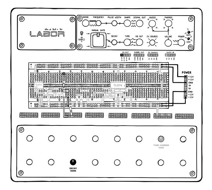
To test this, we'll use LABOR's manual gate, which has a dedicated setting for generating triggers. If you now push the button, you should get a percussive sine wave hit.
