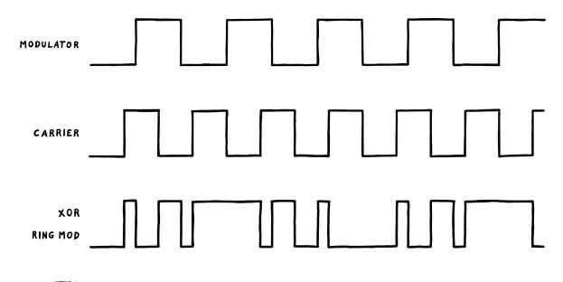
Coincidentally, this signal is identical to what you would get from a ring modulator. Which is why XOR gates are often used as a cheap substitute for true ring modulation. (The Korg MS-20 is one famous example.) To implement an XOR gate, we only need 4 diodes, 2 resistors and a PNP transistor.
