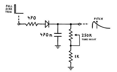
When we apply a trigger to the input, the capacitor gets charged with a very slight delay, making the rising edge less steep. Then, the cap discharges just like it did in our previous envelope. By sending the output to the VCO's control voltage input, we force its pitch to quickly rise and then drop back down. This is a basic simulation of what a beater hitting a drum would sound like. And because an instant rise sounds too aggressive and artificial, we add the small resistor before the cap.
