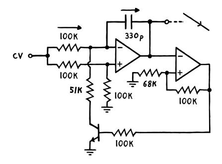
This way, the voltage on the left will stay at half of the CV, while the voltage on the right will steadily drop. This keeps going until the integrator's output crosses the schmitt trigger inverter's lower input threshold, causing it to latch into the high state.
