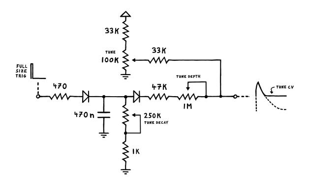
Also, we'll set up another diode after the envelope's output – so that it only affects the total mix if the envelope is higher than the tune CV. **This way, we will always drop down to the set base pitch (and not lower)**. For the trigger, we'll use the unaccented one again, since the pitch bend is integral for the output to sound like a drum. Making it less noticeable on an un-accented hit doesn't sound quite right to me (though maybe it does for you – give it a shot!).
