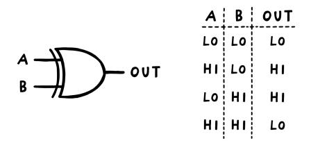
If either input is high while the other is low, the XOR's output will be high. But if both inputs are the same value, its output will be low. With two dissonant square waves as our inputs, this creates a pulse wave with semi-chaotic pulse width that sounds harsh and metallic.
