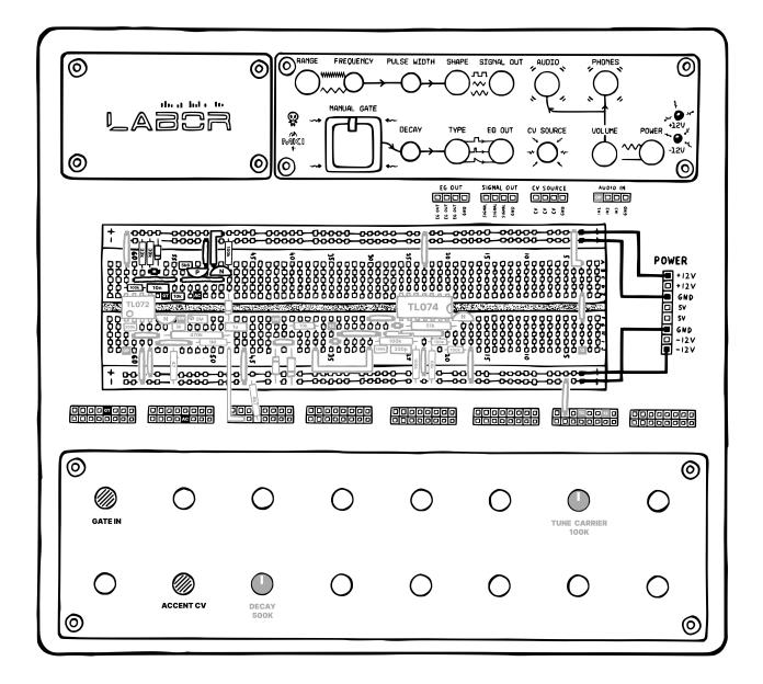
To test this, connect a sequencer to both the gate input and the accent CV input. (Alternatively, you can also use LABOR's EG OUT socket and the CV SOURCE.) You should be able to trigger the circuit and set its output volume simultaneously.
