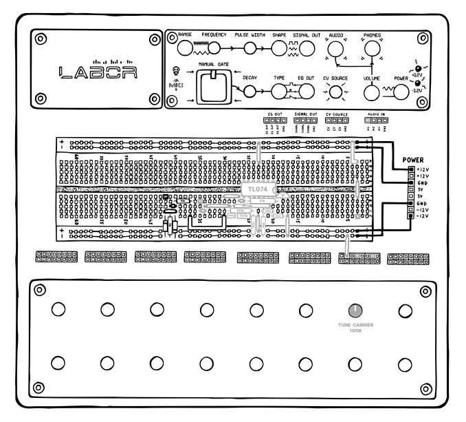
For our triangle wave, the amount of scaling is just right: the waveshaper should give you a pretty decent sine wave on the oscilloscope that's noticeably less buzzy.<sup>3</sup>
