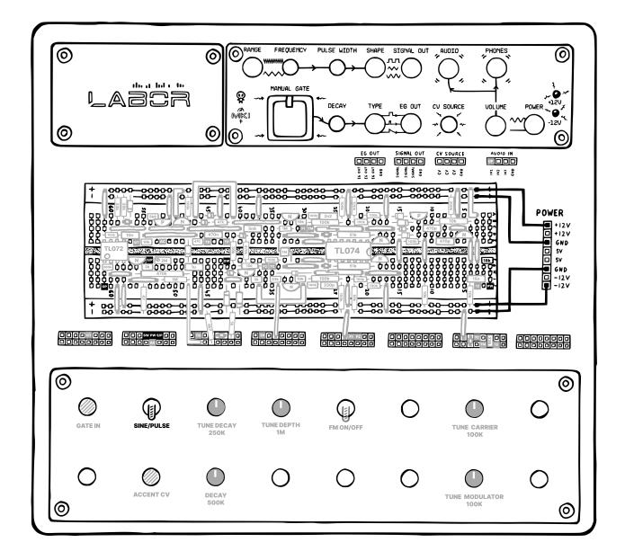
To test this, first set the VCA's input to pulse wave and turn the FM mode off. By tuning the two oscillators to different intervals, you can get a decent variety of cymbal- and hihat sounds. Cool – but what if you also turn on the FM mode? The difference is subtle, but you should get a different *flavor* of cymbal.
