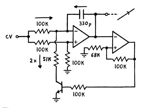
Which, conveniently, is exactly as much as is flowing in from the CV. **Causing the integrator's output to rise at the same rate it was previously dropping at**. Until it hits the schmitt trigger inverter's upper input threshold, and the whole cycle repeats.
