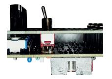
The switches need special attention. Insert the **switches** in relevant places, but **do not solder** them, yet. Place the front panel, fix it with a potentiometer and jack socket nuts. Then tighten switch nuts, so that switches are pushed against the front panel. Now, solder the switches.
