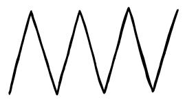
If you don't see any signal at all (or get a constant 0 V output), check if the op amp **DA1** is properly installed. The direction of chip and socket need to be aligned with the direction indicated on the silkscreen. Also check if the resistor **R43** and capacitor **C8** are properly soldered to the PCB.
