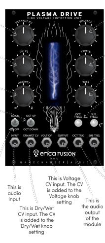
Adjust overdrive level manually from light to extreme in far CW setting. The Voltage CV is added to the knob setting
