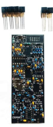
Next, insert and solder **transistors.** There are PNP and NPN transistors in the kit, therefore before soldering them, I highly recommend to sort them. Make sure you install them in correct places and pay attention on the orientation of the transistors – notch on the silkscreen has to match the flat part of the transistor.
