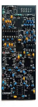
Then proceed with other resistors. Remember – if you are not sure about resistor values, use the multimeter to check! When al resistors are installed, your Hi-Hats PCB should look like this:
