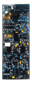
Also, populate the 1 uF film capacitor and **2x5 PSU socket.** Make sure the orientation of the socket is as shown in the picture below – the arrow pointing to the first pin is aligned with a notch on the silk-screen. The key on the socket will be facing down the PCB. Now your PCB should look like this:
