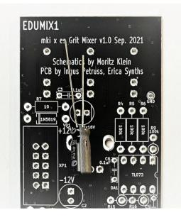
Now **insert & solder the electrolytic capacitors.** Electrolytic capacitors are bipolar, and you need to mind their orientation. The positive lead of each electrolytic capacitor is longer, and there is a minus stripe on the side of the capacitor's body to indicate the negative lead. On our PCBs, the positive pad for the capacitor has a square shape, and the negative lead should go into the pad next to the notch on the silkscreen.
