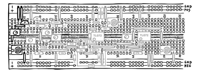
You can test this by sending a CV signal from your sequencer into the new pitch CV input. Of course this simplistic implementation does not adhere to the volt per octave standard – but I think it's pretty useful regardless.
