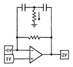
And this would continue until the op amp runs into the upper supply voltage – if it weren't for the bridge resistor between output and inverting input. Because as the op amp pushes harder and harder, that resistor allows a small current to charge up the second cap from the other side.
