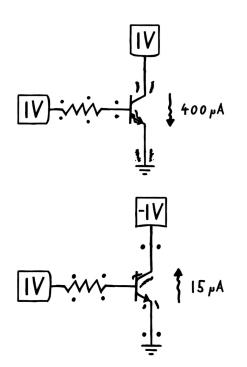
Let's imagine we isolate our transistor and apply 1 V to the base via a 100k resistor, 1 V to the collector and 0 V to the emitter. This will cause around 400  $\mu$ A to flow between collector and emitter in what we call the transistor's forward active mode.
