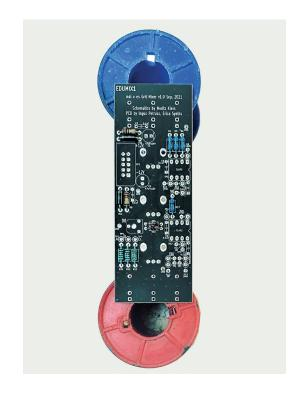
Place the Kick Drum PCB in a PCB holder for soldering or simply on top of some spacers (I use two empty solder wire coils here).
