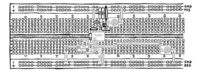
If you now feed your gate signal into the gate-to-trigger converter, you should get a single kick hit instead of two per gate.
