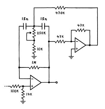
Here's how it works. We'll imagine that we've just triggered the kick, which means that the output voltage is rising. Like before, this will push current out of the first capacitor. But unlike before, we also actively pull current out via this newly added, second path. That's
