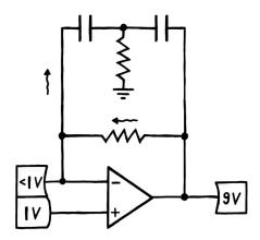
At some point, this process will add more voltage on the left as we lose on the right, causing the whole mechanism to kick into reverse gear. Now, the op amp will start dropping its output voltage to try and course correct. Only problem is that this will pull current out of the first cap, and subsequently up from ground, increasing the voltage between the two caps and also at the inverting input. Which forces the op amp to reduce its output voltage even further.
