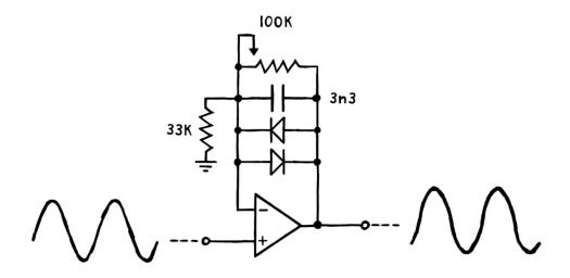
That's because the cap allows very quick changes in the op amp's output voltage to pass through to the inverting input – while slower changes (i.e the majority of the kick's waveform) get blocked. We're effectively adding a low pass filter whose cutoff frequency is determined by the size of the cap. So a smaller cap gives us more overtones and harshness, while a bigger cap gives us less.<sup>15</sup>
