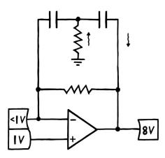
Eventually, we'll again reach a tipping point where the whole mechanism reverses. Only this time, it'll be at a slightly lower output voltage. **That's because with every charging and discharging cycle, we lose a bit of the momentum we initially put in**. The circuit behaves kinda like a pendulum that way.
