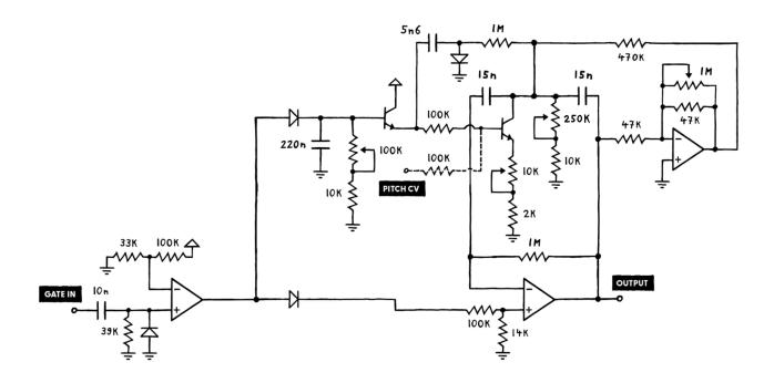
Well, if you'd try this, you'd quickly notice that it doesn't sound too great: the pitch envelope loses some of its punch, and it slides upwards weirdly. What's up with that? Well, the problem is that our CV input is competing with the envelope generator, as both are trying to set the oscillator's pitch directly. This means that neither can do their job properly. To fix it, we need to make them work together. Here's how.
