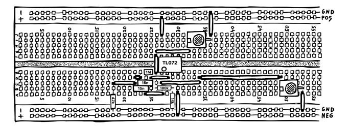
You should get a quick, low-frequency bump when the gate goes high. Great! Though you might also notice a second bump when the gate goes low. What's up with that? Well, as we saw earlier, the oscillation is triggered when the voltage at the non-inverting input changes and the op amp struggles to charge (or discharge) the second cap to that voltage. So it makes sense that we get a second bump when the input voltage drops.
