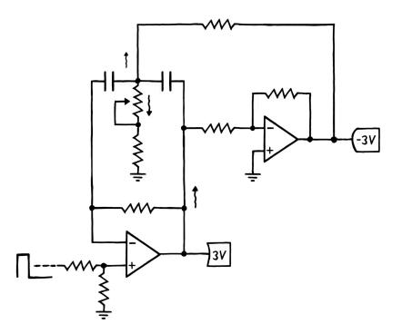
And of course, the same idea applies in reverse when the kick's output drops below 0 V. Then, the inverting buffer will push against the caps, exaggerating the downward motion of the kick. **We're basically applying positive feedback to the system**. Which, with the resistor values specified above, will keep the oscillation going indefinitely without altering the pitch.
