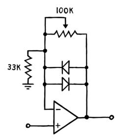
Here's how it works. If the potentiometer is dialed all the way down, there is a direct, unimpeded connection between the op amp's output and inverting input, which turns it into a straight buffer. So it simply replicates the signal applied to the non-inverting input. But as we dial that pot up, things get interesting. Because now, the two resistances form a voltage divider. Which, by itself, would simply increase the op amp's gain and therefore the output volume.
