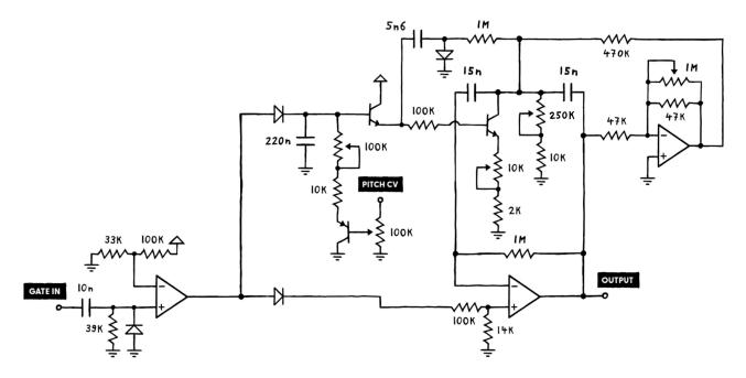
That's because that PNP only passes current between emitter and collector if the emitter voltage is higher than the base voltage. Once they're (almost) the same, the current flow will stop. Now, to give ourselves some control over how strongly the pitch CV affects the kick, we'll route that CV through a variable voltage divider. That way, we can dial in any ratio between 0 and 1.
