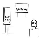
**A bunch of capacitors**. The specific values (which are printed onto their bodies) are
