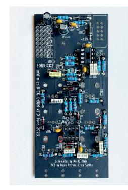
Next, insert and solder **transistors.** There are PNP and NPN transistors in the kit, make sure you install them in correct places and pay attention on the orientation of the transistors – notch on the silkscreen has to match the flat part of the transistor.
