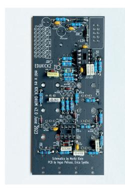
Then proceed with the **ceramic and film capacitors.** Place the PCB in your PCB holder or on spacers, insert the capacitors and solder them like you did with the resistors & diodes before. Now your PCB should look like this:
