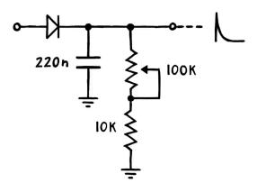
It works like this. If we apply our trigger to the input diode, current will flow into the 220 nF capacitor, instantly filling it up. Then, when the voltage pulse disappears, the charge inside the cap will drain out via the resistance to ground. At the output node, this will result in a gradually falling voltage curve – with its steepness depending on the resistance we dial in using the potentiometer. Great! But before we can send this into our transistor, we need to isolate the output node.
