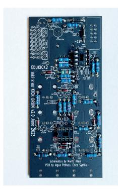
**Next, insert the first DIP socket**, hold it in place and solder one of the pins. Continue with the **next DIP socket**. Make sure the DIP sockets **are oriented correctly** – the notch on the socket should match the notch on the PCB's silkscreen. Now, turn the PCB around and solder all remaining pins of the DIP sockets.
