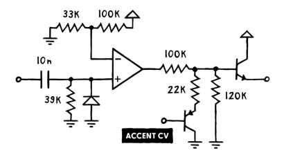
That's because the added resistance creates a secondary voltage drop before the **PNP's emitter**. So the bigger that resistor, the more we raise the minimum voltage level above it. When testing this, I found that a 22k resistor works best here – resulting in a 2 V spike at the output when the accent CV is 0.
