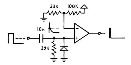
When we apply a gate signal to the input capacitor, we get a voltage spike on the other side that quickly dies down as the cap charges through the 39k resistor to ground. For the split second this spike crosses its threshold voltage, the comparator will then push out an extremely short 12 V gate – also called a trigger. (Those 12 V are then scaled down to around 1.4 V by the voltage divider at our kick's trigger input.)
