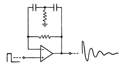
So let's look at how this works.<sup>4</sup> We'll assume that the voltage at the op amp's noninverting input quickly jumps from 0 to 1 V. Now, to reach a state of balance, the op amp will try to push the voltage at its inverting input up to 1 V as well. For that, it'll increase its output voltage to 1 V. Initially, this will work just fine, since that voltage pushes straight through the two capacitors and reaches the inverting input that way.
