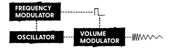
Alright, this should be everything we need. So let's think about how we could implement these blocks in our circuit. In an ideal scenario, we'd want to use a full blown VCO as our oscillator, so we can precisely manipulate its pitch via a control voltage coming from an envelope generator.
