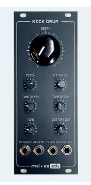
Finally fit the Decay potentiometer knob and we are done!
