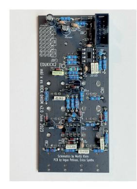
Then complete the component side of the Kick Drum PCB by soldering the **PSU socket.** Make sure the orientation of the socket is as shown in the picture below – the arrow pointing to the first pin is aligned with a notch on the silkscreen. The key on the socket will be facing outwards the PCB. Now your PCB should look like this:
