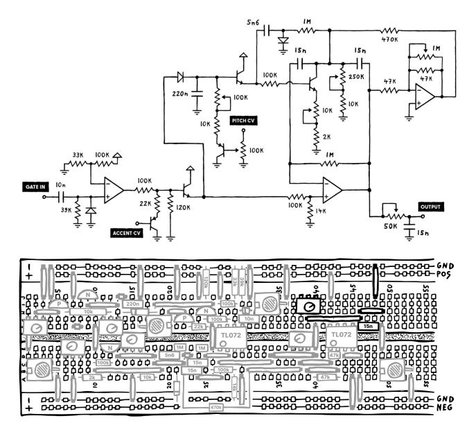
And while is going to work in principle, the volume will drop significantly as you lower the cutoff. This is because the passive low-pass affects the circuit's output impedance. So we'll simply buffer it, right? Well, yeah – but we can actually do one better.
