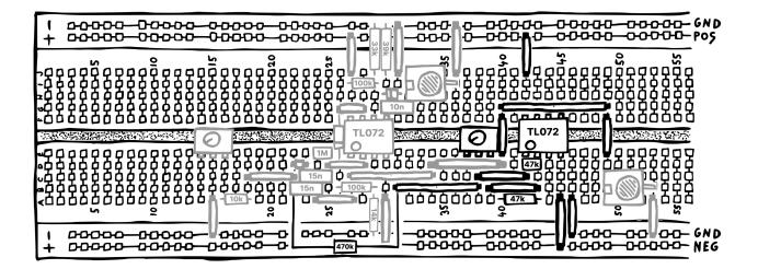
If you test this, you'll notice that dialing in the decay goes from short to long very smoothly. What's even better is that the kick doesn't go into full drone mode at the maximum setting. That's because two resistances in parallel will always net you a lower total resistance than either individually.
