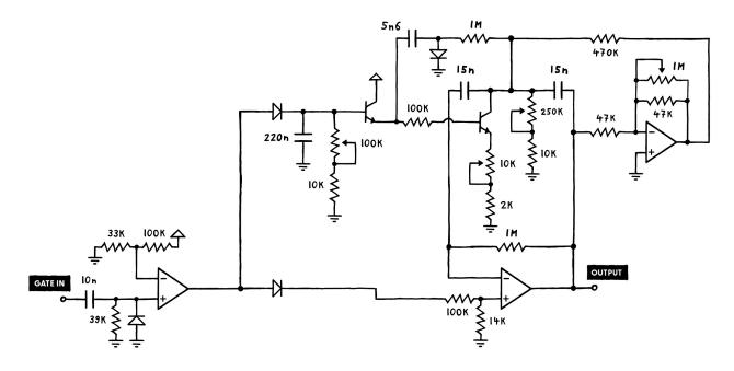
Here's how it works. When our envelope is triggered, the buffer transistor pushes a burst of current into the newly added cap. (This is possible because the diode allows current to flow to ground on the other side.) Next, when the envelope's output voltage drops, that new cap won't immediately discharge into the oscillator's CV input. That's because current can't flow back up from ground and into it from the other side.
