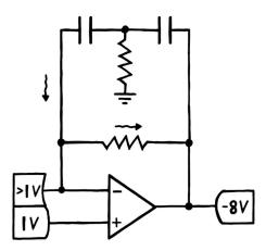
And so the output it produces is a sine wave swinging around the non-inverting input voltage with a steadily decreasing amplitude. Which should already sound pretty kick drum-ish – if the frequency is low enough. To make sure that it is, we have to choose the right combination of capacitor and resistor values. This is a little tricky, since all of those values influence both frequency and decay at the same time.
