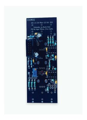
Then complete the component side of the Mixer PCB by soldering the **PSU socket and multiturn trimmer potentiometer**. Make sure the orientation of the socket is as shown in the picture below – the arrow pointing to the first pin is aligned with a notch on the silkscreen. The key on the socket will be facing inwards the PCB. Now your PCB should look like this:
