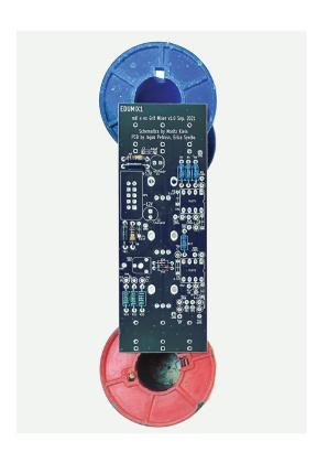
Place the VCF PCB in a PCB holder for soldering or simply on top of some spacers (I use two empty solder wire coils here).
