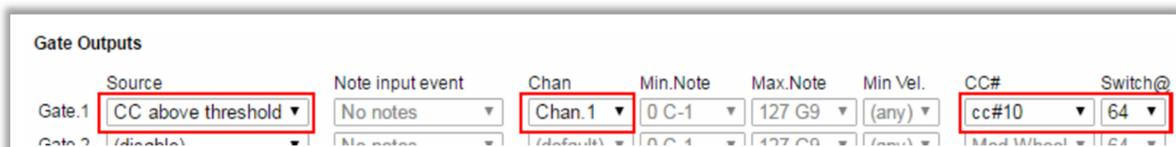
We can also set a gate to trigger when a CC is below a threshold. In all cases the gate cannot trigger until we receive the current value of the CC from MIDI (i.e. when we first connect Mutant Brain we don't know the current CC value until it changes).
