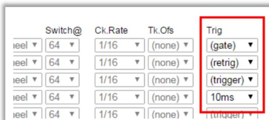
The trigger period in global settings applies only to trigger mode. In retrig mode the “low” time is very short (~1ms) and just enough to give a rising edge to trigger your synth gear.
