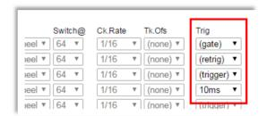
The trigger period in global settings applies only to trigger mode. In retrig mode the "low" time is very short (~1ms) and just enough to give a rising edge to trigger your synth gear.
