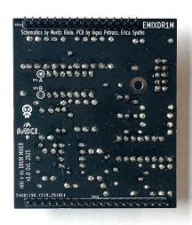
Now, turn the PCB around and inspect your solder joints. Make sure all components are soldered properly and there are no cold solder joints or accidental shorts. Clean the PCB to remove extra flux, if necessary. Then insert the male connectors and solder those. The completed Main PCB has to look like this:
