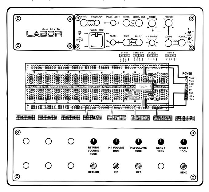
Try connecting the send output to an effect and routing its output back to the return input. You should now be able to apply the effect only to specific channels by adjusting their send potentiometers.
