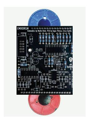
Let's start assembly with the Main PCB! Place the **Output Mixer 2 PCB in a PCB holder for soldering** or simply on top of some spacers (I use two empty solder wire coils here).
