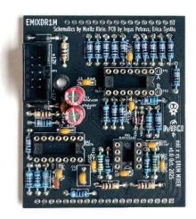
Then populate the **2x5 PSU socket**. Make sure the orientation of the socket is as shown in the picture below – the arrow pointing to the first pin is aligned with a notch on the silkscreen. The key on the socket will be facing inwards the PCB. Now your PCB should look like this:
