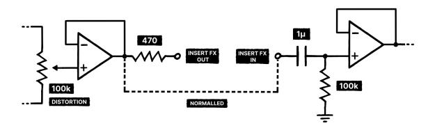
Here's how it works. The mixed and distorted signal is sent to the INSERT FX OUT jack, where it can be patched into an effect like the compressor or BBD. The processed signal then returns through the INSERT FX IN, which feeds directly into the high-pass filter at the start of our output stage.
