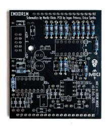
I usually start populating PCBs with lower, horizontally placed components, resistors specifically. There are lot of 100k resistors, so let's start with those! Bend the resistor leads and insert them in the relevant places according to the part placement diagram above. Flip the PCB over and solder all components. Then, use pliers to cut off the excess leads.
