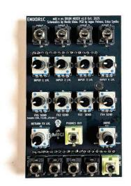
Now, insert the potentiometers in relevant places, but **do not solder** them, yet! There are 9 A100k potentiometers, and one B100k potentiometer (DRIVE). Make sure, you don't mix the values.
