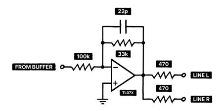
A small 22 pF capacitor across the feedback resistor keeps it stable, and both sides of the stereo output jack are driven from this single op amp through 470 ohm resistors. To avoid cluttering the breadboard unnecessarily, we'll only set up one headphone output stage – you've already seen firsthand how a regular op amp drives low impedance loads.
