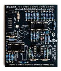
Next, insert the first **DIP socket**, hold it in place and solder one of the pins. Continue with other DIP sockets. Make sure **the DIP sockets are oriented correctly** – the notch on the socket should match the notch on the PCB's silkscreen. Now, turn the PCB around and solder all remaining pins of the DIP sockets. Compare your socket placement with the one on the picture below.
