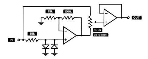
Here's how it works. We take both the dry and the distorted signals and connect them to opposite sides of a 100k potentiometer. The wiper in the middle gives us a mix of the
