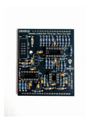
Then proceed with the ceramic capacitors. Start with soldering 0,1uF capacitors - place the PCB in your PCB holder or on spacers, insert the capacitors and solder them like you did with the resistors & diodes before then proceed with other ceramic and film capacitors. When completed, your PCB should look like this:
