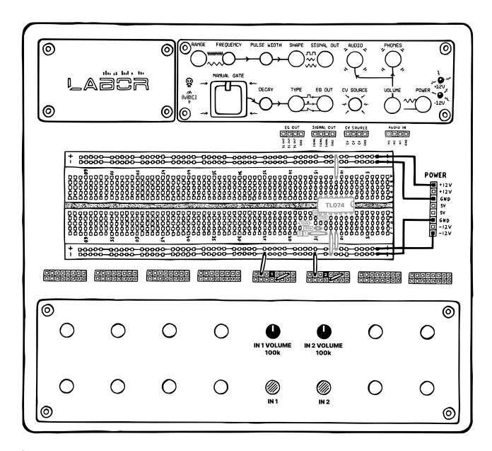
Once you've set this up, try connecting audio signals to both inputs and play with the two potentiometers. You should be able to smoothly adjust the volume of each channel.
