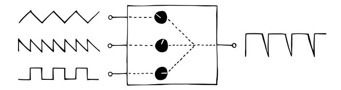
In our case, we want to mix 4 signals: Kick Drum, Hi-Hat, Snare Drum, and FM Drum. The resulting drum mix should then be made available via a single output. Ideally, we'll also want to adjust the individual volume levels for every input signal. Okay, so how do we do that?
