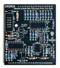
Now, proceed with other resistors, switching diodes and the power protection diodes. Remember – when inserting the diodes, orientation is critical! A thick white stripe on the PCB indicates the cathode of a diode – match it with the stripe on the component. Solder all diodes.
