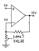
How about amplifying a signal though? To do that, we'll have to turn our buffer into a proper non-inverting amplifier. We can do that by replacing the straight connection between inverting input and output with a voltage divider, forcing the op amp to work harder. Here's how that works. Say we feed our non-inverting input a voltage of 5 V. Now, the output needs to push out 10 V in order to get the voltage at the inverting input up to 5 V. We call this setup a non-inverting
