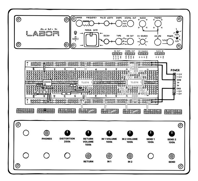
Try connecting a pair of power-hungry headphones to the new output (bottom left) – you should get a clean, solid signal at proper listening level. With the output stage complete, the signal path is now done – and we can turn our attention to one final feature: insert effects.
