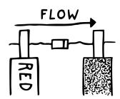
In some cases, it doesn't matter which probe you connect to which component leg or point in your circuit. This is true for testing resistors, non-polarized capacitors (foil/film, ceramic, teflon, glass etc.), continuity<sup>18</sup> or AC voltage.
