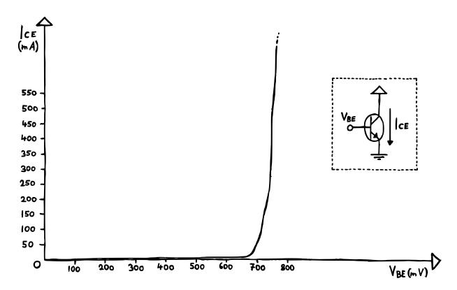
First, the relation between base voltage and collector current is exponential. Second, unlike a resistor, a BJT is not symmetrical – so we can't really reverse the direction of the
