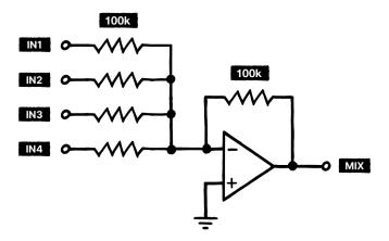
Here's how it works. The op amp is wired so that its inverting input (-) stays as close to 0 V as possible. That's because the circuit only reaches a state of balance when the voltage at the inverting input matches the voltage at the non-inverting input (+). So whenever the inverting input moves away from 0 V, the op amp adjusts its output in the opposite direction to restore balance.
