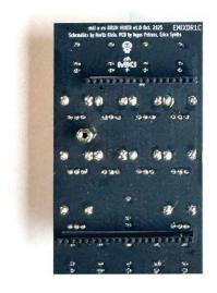
Next, fit the front panel, screw some nuts on the jack sockets and make sure that the potentiometer shafts are aligned with the holes in the panel – and that they're able to rotate freely. Now, go ahead and solder the potentiometers and then remove the front panel. Then use the M3 screw to fix the 11mm spacer – it will fix both PCBs together and secure integrity of the module.
