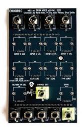
Next, proceed with the Controls PCB. Insert all **jack sockets** and solder them. Please, note that two jack sockets are **stereo**. They are **green**, and their pinout is identical to mono sockets, so make sure you solder them in correct places.
