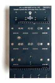
Turn the Connectors PCB around and solder the **female connectors!**
