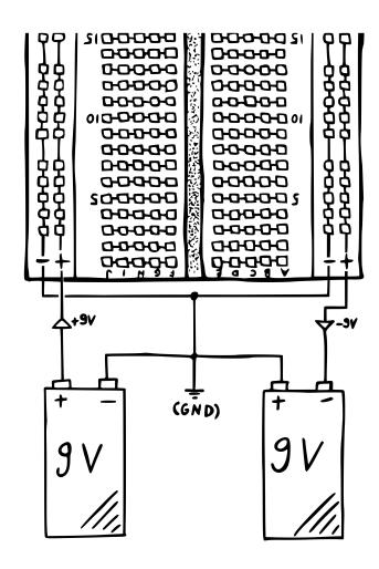
By connecting the batteries like this, the positive terminal of the left battery becomes your +9 V, while the negative terminal of the right is now your -9 V, and the other two combine to become your new ground.<sup>10</sup> **Please make sure you disconnect the batteries from your breadboard when you make changes to the circuit!** Otherwise you run the risk of damaging components.
