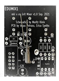
Now, insert & solder the electrolytic capacitors. Electrolytic capacitors are bipolar, and you need to mind their orientation. The positive lead of each electrolytic capacitor is longer, and there is a minus stripe on the side of the capacitor's body to indicate the negative lead. On our PCBs, the positive pad for the capacitor has a square shape, and the negative lead should go into the pad next to the notch on the silkscreen.
