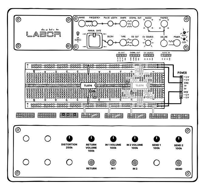
After setting this up, try dialing in different distortion levels. You should hear the character of the distortion change smoothly from subtle warmth to full-on grit – while the overall volume stays the same.
