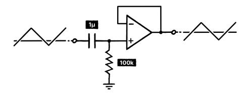
Together, these form a high-pass filter with a cutoff around 1.6 Hz – low enough to remove DC and sub-audio content without affecting the audible range. To prevent loading effects, we buffer this stage with another op amp before processing the signal further.
