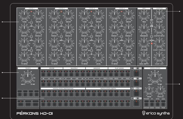
The Master section includes a built in BBD emulation with time and feedback controls, as well as a dedicated modulation LFO for the delay time. The Delay can be either synchronized to the clock or free-running, depending on the configuration.
