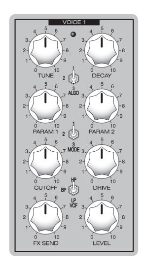
The **PARAM1** and **PARAM2** knobs control different parameters depending on the algorithm selected. Please, refer to the table below.
