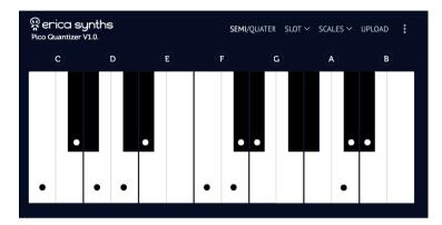
THE PICO QUANT PICO QUANT SCALE DESIGN INTERFACE ALLOWS YOU TO DESIGN YOUR OWN UNIQUE SCALES WITH 1/4 SEMITONE ACCURACY OR SELECT ONE OF 16 PREDEFINED SCALES. FOLLOW SIMPLE STEPS TO DESIGN AN UPLOAD SCALES TO THE MODULE!
