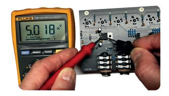
If voltage reads something around 5 volts, you are good to install the RP board. Disconnect a power supply and **install the RP board.** Once it's installed, power the unit on and make sure, the LEDs on the **cherry keys lit up sequentially and the LEDs on the RP board are on.**
