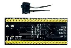
In order to ensure correct operation of the instrument, you need to solder two "jumpers" on the RP board. Just put the solder blob on smt polygons indicated in the picture.
