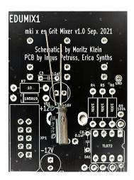
Also, **install the voltage regulator** (LDO) – bend it's leads and solder it in place. The LDO will disperse all heat generated in the process of lowering the voltage. Before soldering, make sure, the LDO touches a heatsink on the PCB (no big deal, if it doesn't because not that much heat is generated). Also **install and solder remaining 1k vertically placed resistor.** When completed, your PCB should look like this:
