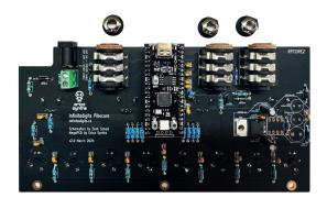
Now you can **insert the PCB in the enclosure.** Make sure the DC connector clicks in the relevant opening and **washers of the jack sockets touch rear panel.** Tighten jack socket hex nuts and then **fix the PCB with 3 screws** in a cherry key area.
