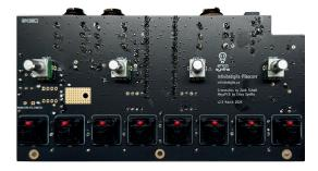
Cut a wire in the kit in two pieces and solder it to the **power switch.** Also, solder the **male connectors to the RP board.** Start with one pin, make sure a connector is aligned with the silkscreen and is positioned vertically. Do not install these components, yet.
