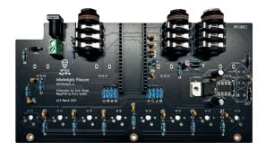
Now, turn the PCB around and inspect your solder joints. **Make sure all components are soldered properly and there are no cold solder joints or accidental shorts.** Clean the PCB to remove extra flux, if necessary.
