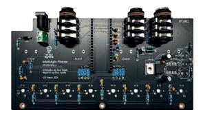
Now turn the PCB around and inspect your solder joints. Make sure all components are soldered properly and there are no cold solder joints or accidental shorts. Clean the PCB to remove extra flux if necessary. Now let's proceed with the cherry keys! Each key has an LED inside, and the orientation of the LED is critical. The longer lead is the anode and all LEDs have to be aligned with the PCB as shown below.
