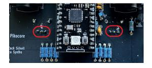
2. Solder a wire from the center pins of potentiometers to the pin 27 and pin 28 of the RP board as shown on the picture.
