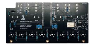
Now, we recommend sorting the ceramic capacitors. There are 100nF, 10nF and 1uF ceramic capacitors in the kit. 100nF have 104, 10nF have 103, and 1uF has 105 printed on the capacitor. Start by populating the 100nF capacitors.
