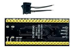
In order to ensure correct operation of the instrument you need to solder two "jumpers" on the RP board. Just put the solder blob on the smt polygons indicated in the picture.
