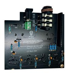
Measure voltage between pins 2 and 3 of the LDO.
