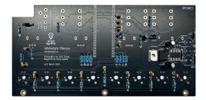
Now, solder all jack sockets and connectors. Make sure all components are properly pushed in the relevant places and the connectors are aligned with the silkscreen and vertical. We recommend soldering one pin of the component and double-checking the alignment. Also, solder the two-pin male connector for the jumper next to the XS3 jack socket. If you will use a mono jack for the audio output, do not install the jumper. At this stage your PCB should look like this:
