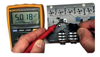
If the voltage reads somewhere around 5 volts, you are good to install the RP board. Disconnect the power supply and install the RP board. Once it is installed, power the unit on and make sure that the LEDs on the cherry keys light up sequentially and the LEDs on the RP board are on.
