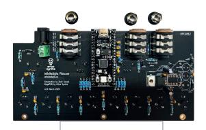
Now you can insert the PCB into the enclosure. Make sure the DC connector clicks into the relevant opening and that the washers of the jack sockets touch the rear panel. Tighten the jack socket hex nuts and then fix the PCB with 3 screws into the cherry key area.
