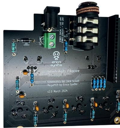
Measure **voltage** between pins 2 and 3 of the LDO.
