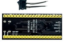
At this point it's a good idea to test if the voltage regulator works. Use one excess lead of a resistor to emulate a closed switch and connect the power supply.
