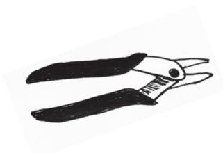
**Cutting pliers.** Use them to cut off excess component leads after soldering.
