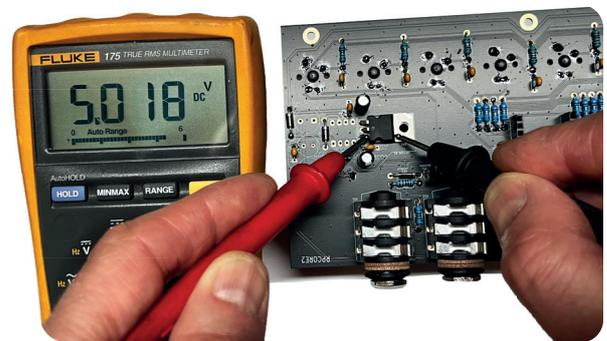
If the voltage reads somewhere around 5 volts, you are good to install the RP board. Disconnect the power supply and install the RP board. Once it is installed, power the unit on and make sure that the LEDs on the cherry keys light up sequentially and the LEDs on the RP board are on.
