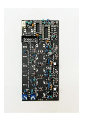
Then complete the component side of the Envelope PCB by soldering the **PSU socket** and **trimmer potentiometers**. Make sure the orientation of the socket is as shown in the picture below – the arrow pointing to the first pin is aligned with a notch on the silkscreen. **The key** on the socket will be **facing down**. Now your PCB should look like this:
