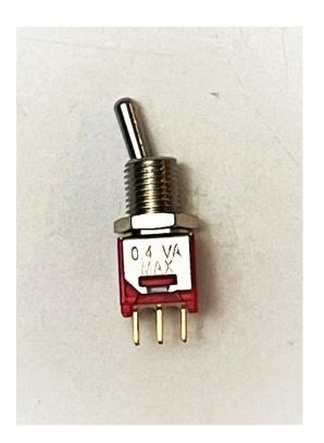
The **switches** require special attention. There are two nuts for the switch (they look identical to the jack socket nuts, but the thread is different). Screw on one of the nuts until it fixes itself on the bottom of the thread.
