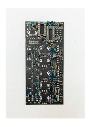
Next up: inserting & soldering transistors. Make sure you align the transistor with the marked outline on the silkscreen – orientation is critically important here.
