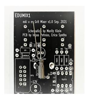
Now, insert **film capacitors** and solder them. Then, insert & solder **the electrolytic capacitors**. Electrolytic capacitors are bipolar, and you need to mind their orientation. The positive lead of each electrolytic capacitor is longer, and there is a minus stripe on the side of the capacitor's body to indicate the **negative lead**. On our PCBs, the positive pad for the capacitor has a square shape, and the negative lead should go into the pad next to **the notch** on the silkscreen.
