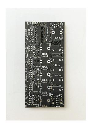
Now, turn the PCB around and inspect your solder joints. Make sure all components are soldered properly and there are no cold solder joints or accidental shorts. Clean the PCB to remove extra flux, if necessary.
