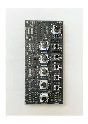
Insert **the potentiometers** (make sure, you have right values! The RATE potentiometer is 250 kOhm, step potentiometers are 100 kOhm), **but don't solder them yet**! Fit the front panel (you may want to fix it with few nuts on the jack sockets) and make sure that the potentiometer shafts are aligned with the holes in the panel – and that they're able to rotate freely. Now, go ahead and solder the potentiometers.
