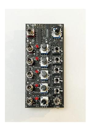
Insert the LEDs in the relevant places on the PCB, but do not solder them, yet! Orientation of the LED is important – check the silkscreen! A notch on the silkscreen indicates the **cathode of the LED** (a shorter lead next to a notch on the LED) and the longer lead – the **anode of the LED** – has to go into a hole with square-like polygon on the PCB.
