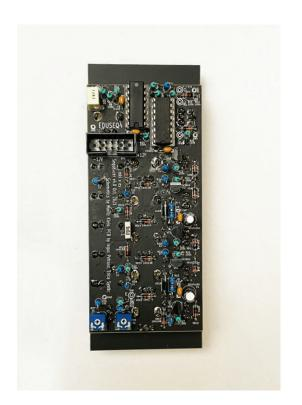
Now, insert the ICs into their respective DIP sockets. Mind the orientation of the ICs – match the notch on each IC with the one on its socket.
