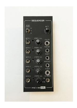
Now, insert **the switches** in the relevant places on the PCB, place the front panel, fix it with few nuts on the jack sockets and **solder the switches**.
