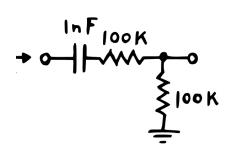
Now, by placing a resistor after the capacitor, we give that path a default resistance – just like we've done for the shelf filter. The effect is different, though. Instead of letting a baseline amount of high frequencies pass through, we set an upper volume limit for them. **That's because where before, high frequency oscillations could pass through the cap as if it wasn't even there, now, they have to fight the additional resistance**.<sup>23</sup>
