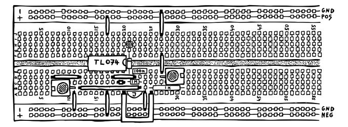
To see if everything works as expected, connect a slow oscillation (e.g. from a looped envelope with long attack & release times) as your to-be-sampled signal. Next, hook up a jumper to the diode at the marked spot. This way, you can easily trigger the sample-and hold-phases by plugging the other end into the positive or negative rail.
