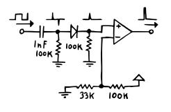
To do that, we just need a simple high pass filter, which is really only a capacitor followed by a resistor to ground. This will convert our square wave into two voltage spikes – one positive, and one negative. To make those spikes really short and snappy, I'm using a super small 1 nF capacitor and a big 100k resistor.
