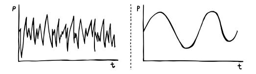
In these diagrams, we draw pressure in a medium over a given period of time. This way, we get what you'd usually refer to as the sound's waveform. For our sine wave (on the
