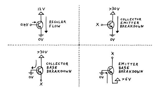
What does this mean? **Simple: it means that you can only push the transistor so far before it starts misbehaving**. If we apply more than 30 V between collector and emitter, for example, the transistor will start to conduct even when it normally shouldn't.
