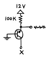
Now, to actually make noise happen, we only need two components: the transistor and a resistor. Here's how it works. We connect our transistor's emitter to the positive supply voltage through a resistance. Then, we ground the transistor's base while leaving the collector unconnected.
