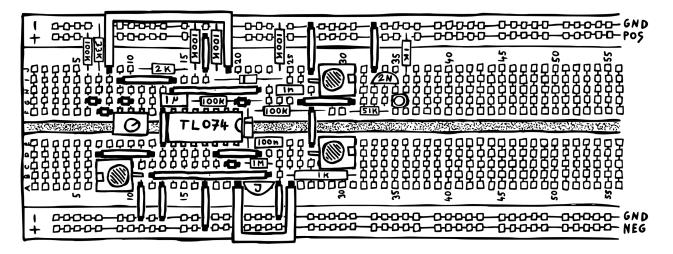
Once you've set this up, try plying around with the clock generator's potentiometer. You should see the status LED flash slower or faster, depending on the amount of resistance you dial in. Also, the sample & hold-circuit should do its thing in sync with that status LED. If you want, you can also test plugging in an external trigger source.
