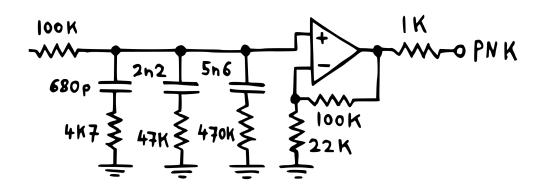
Here's how it works. As we've seen before, the amount of resistance between the capacitor and ground in relation to the input resistance will determine the amplitude at which the individual slope straightens out. Similarly, the size of the capacitor will determine the point at which it starts dropping off – just like in a regular low pass. Knowing this, we can select our component values so that all three slopes affect different parts of the frequency spectrum.
