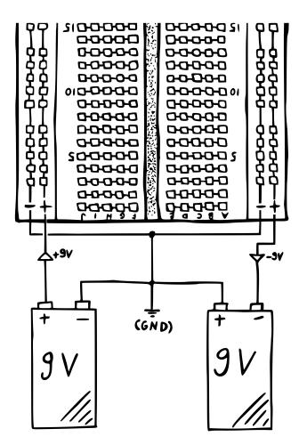
By connecting the batteries like this, the positive terminal of the left battery becomes your +9 V, while the negative terminal of the right is now your –9 V, and the other two combine to become your new ground.<sup>25</sup> **Please make sure you disconnect the batteries from your breadboard when you make changes to the circuit!** Otherwise you run the risk of damaging components.
