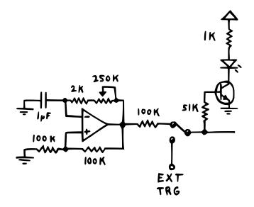
As we've just learned, the clock will swing between +12 V and -12 V. Connected straight to the high pass at the trigger input, this would result in massive ~23 V spikes. To calm those down a bit, we'll simply put a 100k resistor between the clock generator's output and the trigger input. This will limit the amount of current flowing into and out of the capacitor there, cutting the spikes down to just around 8 V.
