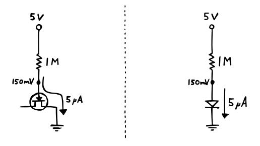
So as long as the voltage at the top is 0 V or below, that diode is blocking. But as soon as we go positive, it will start to conduct. And that conductivity ramps up exponentially as the voltage increases linearly. So, simplified: the more we push from above, the quicker and wider the diode will open up, sinking most of the current we manage to squeeze through that ginormous resistor.
