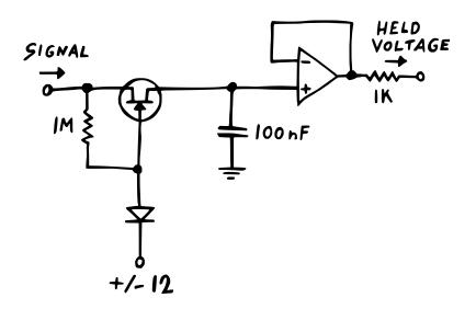
With all this in mind, here's how I decided to set the core circuit up. For now, the input signal is going straight into the JFET. On the other side, I've settled on a 100 nF capacitor. This is big enough to avoid obvious droop, but also small enough to have at least some degree of accuracy.
