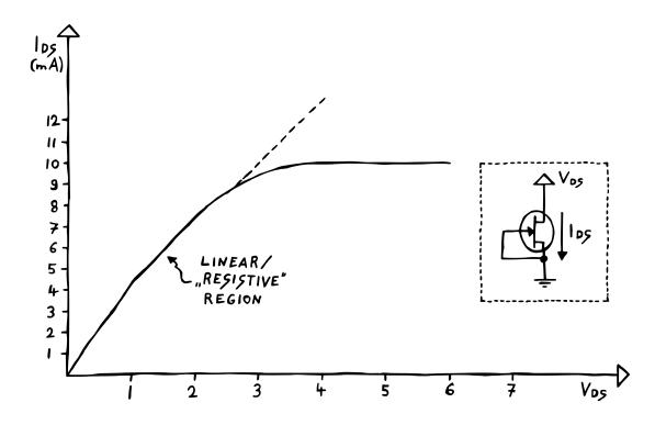
Here, we can see the relation between drain-to-source voltage and drain-to-sourcecurrent, if the gate-to-source voltage stays at 0 V. So: source and gate are fixed at 0 V, while we push up the drain voltage. **Interestingly – and annoyingly – the JFET stops behaving like a resistor after we increase that drain voltage beyond approximately 3 V**. Because with a resistor, the current would simply keep increasing in a straight line. With our JFET, we run into a hard upper threshold.<sup>9</sup>
