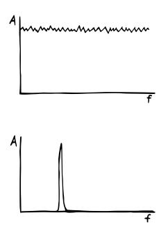
White noise is a noise that occupies the full range of audible frequencies. To illustrate this, we'll check out a simple spectrogram of a white noise signal – where the x-axis is showing frequency, while the y-axis is showing amplitude.
