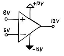
The key here is that op amps are essentially differential amplifiers. This means that they only amplify the difference between their two inputs – not each of them individually. If that sounds confusing, let's check out a quick example. So we'll imagine that one sensor – called the non-inverting input – is reading 8 V from somewhere. The other sensor – called the inverting input – reads 5 V.
