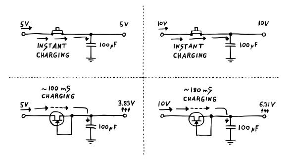
Now if we double the input voltage to 10 V, twice the amount of current has to flow into the capacitor. With our switch, again, that will happen almost instantaneously. With our JFET though, it will take nearly twice as long – since the charging speed stays mostly constant.
