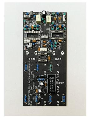
Then complete the component side of the Envelope PCB by soldering the PSU socket. Make sure the orientation of the socket is as shown in the picture below – the arrow pointing to the first pin is aligned with a notch on the silkscreen. The key on the socket will be facing right. Now your PCB should look like this:
