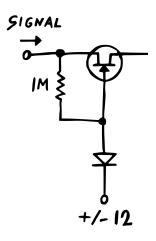
So with this setup, the gate voltage will always be at or close to the source voltage – as long as the diode below the gate doesn't conduct. Why is it here, then? **Simple:** to activate and de-activate the JFET.
