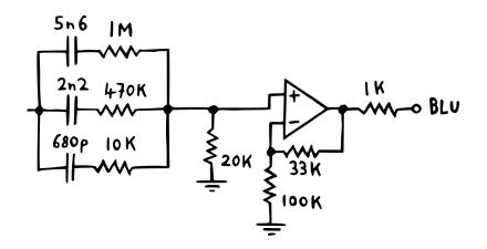
As we now know, the amount of resistance on the input path in relation to the resistance going to ground will determine the amplitude at which the individual slope maxes out – but also the point at which it starts dropping off. The values I've chosen here gave me a result closest to the blue noise examples I found online.<sup>24</sup> Because the filter lowers the overall volume of the noise signal, we'll have to amplify it by a factor of about 1.3.
