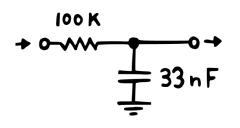
With this in mind, this structure essentially becomes a voltage divider. And in a voltage divider, the output voltage depends on the relation between its two resistors. The weaker the resistance going to ground is compared to the other one, the lower the output voltage will be. And in our scenario here, the capacitor's "resistance" is extremely low, because it's almost empty. Which is why the voltage above it stays close to 0 V.
