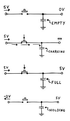
To start out simple, let's take a look at the most naive implementation: using an actual manual momentary switch.<sup>6</sup> Here's how it works. We apply our to-besampled voltage to the switch, while connecting the other end to the capacitor. Before we push down the button, the capacitor will be empty, so the voltage on the right is going to be 0 V.
