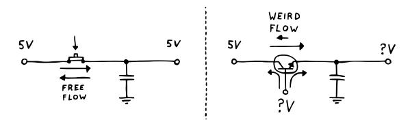
As we know, the transistor will allow for current to flow between its collector and emitter if we apply a voltage to the base. You might then think that applying a voltage to the base is the same as pushing the button on our momentary switch. Only trouble with that is that it's totally not true. A closed switch behaves exactly like a piece of conductive wire. An active BJT does not.
