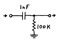
Let's imagine that we use a 2 kHz square wave as the input signal here. Then the amount of current flowing through the capacitor in the wave's high- and lowphases is so small that it never builds up a significant amount of charge.
