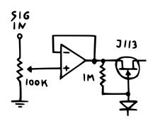
While our circuit is now perfectly usable as it is, we should round it out with a few minor additions. **First, we'll route our signal input through a potentiometer set up as a variable voltage divider.**<sup>17</sup> This way, we can change the input volume on the fly, which might be helpful if we want to reduce the voltage range at the output. Then, we'll buffer the result with another op amp to avoid loading effects.
