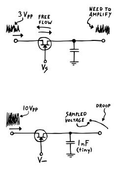
So if we'd scale our input down to 3 V peak-to-peak, then we could charge and discharge our capacitor without that speed limit – which should increase our sampling accuracy quite a bit. The only pain point is that we'd have to also amplify the output signal to get it back up to the original input signal's volume.
