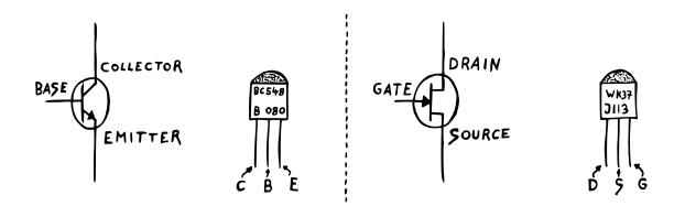
Like the BJT, a JFET (on the right) has three terminals. The naming convention is different, though. Instead of collector, base, and emitter, a JFET has a drain, a gate, and a source terminal. **The flow of current between drain and source is controlled by a voltage applied to the gate**. Since voltages are always just relative, though, we'll have to ask what the point of reference for that gate voltage actually is.
