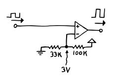
A comparator does just what its name implies: it compares an input voltage to a threshold voltage. Whenever the input is above the threshold, it'll raise its output to the positive supply voltage – and vice versa.
