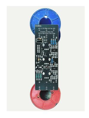
Place the S&H/Noise PCB in a PCB holder for soldering or simply on top of some spacers (I use two empty solder wire coils here).
