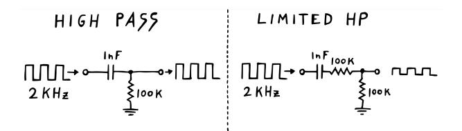
You'll notice that the only difference here is the additional resistor after the input capacitor. To understand the effect this has, let's recap the mechanics of a high pass filter. As the name already implies, a high pass is the exact inverse of a low pass – functionally, but also on the component level.
