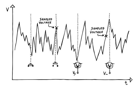
Here's how that would work out in detail. If we activate the JFET in the middle and then de-activate it on the right, the capacitor voltage won't be equal to the then-current input voltage. Simply because there wasn't enough time to get it charged up to that value. **Instead, we'll be getting an output that is somewhat lower**.
