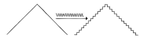
The output then looks like a repeating set of stairs going up and down. **So instead of the continuous slope of the input triangle wave, we get a kind of digital approximation**. If you do this with white noise instead of an LFO, you'll get weird, random voltages at the output instead.
