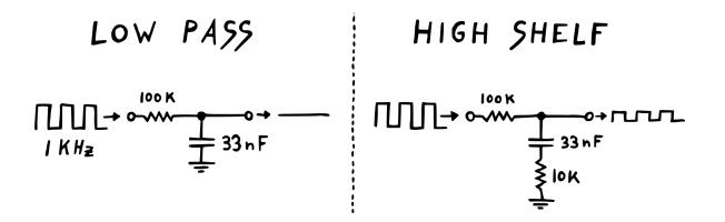
We'll start with a simple high shelf filter. If you compare it to a basic low pass, you'll notice that they're almost identical – save for the additional resistor between the capacitor and ground. To understand why this little change allows a baseline amount of high frequencies to pass through, we'll have to think about the mechanics of a basic low pass filter first.
