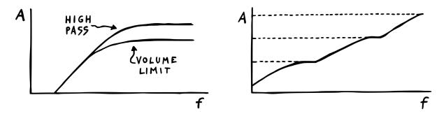
As you can see, they're almost identical – save for the unaffected parts of the signal, which differ in amplitude. Hence the "limited"-idea. Then, just like we've done with the shelf filter before, we can combine multiple of these slopes to create a coarsely stepped 3 dB/octave slope approximation. But first, we'll again have to figure out how a single slope version works. For that, we'll compare it to a basic high pass.
