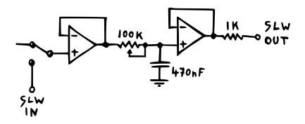
And since you might want to use the slew circuit on some other, external signal, we'll route the sample & hold's regular output through another switched jack socket before sending it into the input buffer.<sup>19</sup>
