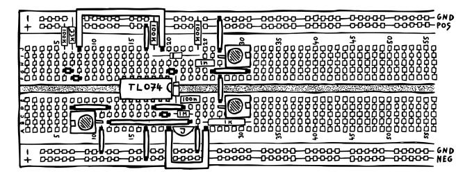
If you now send a square wave oscillation into the trigger input, while connecting the circuit's output to a VCO's CV input, you should hear its pitch go up and down in obvious, distinct steps. Nice – but what if you don't have a square wave LFO at hand? No worries! Since our module should have an internal clock anyways, we'll take slight detour and set one up right now.
