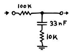
Next, let's imagine we apply the same 1 kHz square wave to the shelf filter with its additional 10k resistor between the capacitor and ground. Where before, the resistance to ground stayed close to 0, now, we've got a default value of 10k ohms. Which, by the law of voltage dividers, must result in a significant output voltage swing. Even with our super high-frequency input and an almost-empty capacitor.
