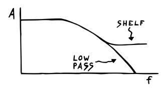
As you can see, they are almost identical – save for how they handle the upper frequency range. Where the low pass cuts off the signal completely after a certain point, the high shelf allows a baseline amount of high frequencies to pass through.
