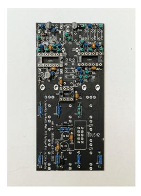
Next up: inserting & soldering the transistors. Make sure you align the transistors with the marked outline on the silkscreen – orientation is critically important here. Also, we have three different kinds of transistors on this module – a BC548 transistor in the noise generator, a 2N3904 transistor in the LED driver for S&H clock rate and a J113 transistor that acts as a switch in the S&H circuit. Pay close attention on the placement of the transistors!
