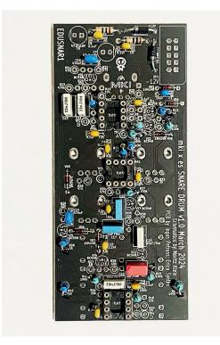
Because the Snare drum features quite few resistors, let's start with **100 k resistors** (light blue on the photo to the left) and **1 k resistors** (dark blue on the photo to the left). When those are installed, the PCB should look like this:
