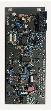
Now, insert the ICs into their respective **DIP sockets.** Mind the orientation of the ICs – match the notch on each IC with the one on its socket.
