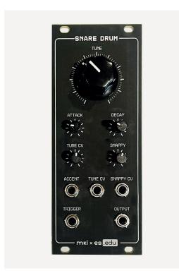
Finally fit the Tune potentiometer knob and we are done!
