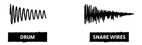
We'll tackle the drum first. For that, we'll rely on the same percussive sine wave oscillator I used in my kick drum circuit. To give it a punchy attack, we'll then modulate its pitch with a simple envelope. For the snare wire sound, we'll start off with a standard white noise generator. Next, we'll use a VCA coupled with another envelope generator to shape the noise into a percussive burst.
