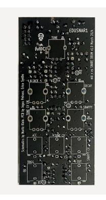
Now, turn the PCB around and inspect your solder joints. **Make sure all components are soldered properly and there are no cold solder joints or accidental shorts.** Clean the PCB to remove extra flux, if necessary.
