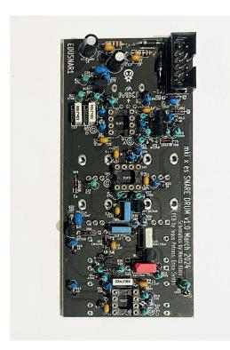
Then complete the component side of the VCF PCB by soldering the **PSU socket.** Make sure the orientation of the socket is as shown in the picture below – the arrow pointing to the first pin is aligned with a notch on the silkscreen. The key on the socket will be facing outwards the PCB. Now your PCB should look like this:
