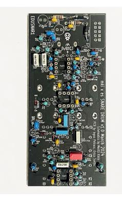
Now, proceed with other vertically placed resistors. If you are not sure about resistor value, use the multimeter to measure resistance of each resistor before soldering them. Once you have completed installing the resistors, your PCB should look like this:
