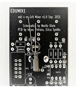
Also, **insert & solder the electrolytic capacitors.** Electrolytic capacitors are bipolar, and you need to mind their orientation. The positive lead of each electrolytic capacitor is longer, and there is a minus stripe on the side of the capacitor's body to indicate the negative lead. On our PCBs, the positive pad for the capacitor has a square shape, and the negative lead should go into the pad next to the notch on the silkscreen.
