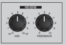
The SYNTRX has two built in speakers for monitoring purposes and experiments with feedback loops. Use the MUTE/ON switches to turn them on or off. At louder settings, the speakers may distort the sound and with spring reverb in action, they will go into feedback loop with the spring. You can use it as a sound source for future treatments. You may also want to try playing feedback loops with a microphone connected to the input and bringing it to the speaker.
