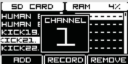
Note that you need to upload samples to both channels 1/2 individually – use the switch to select the channel and upload samples; popup screen will inform you, which channel is currently active. The message in the top right column will indicate RAM usage. Take note that both sides share the same RAM!
