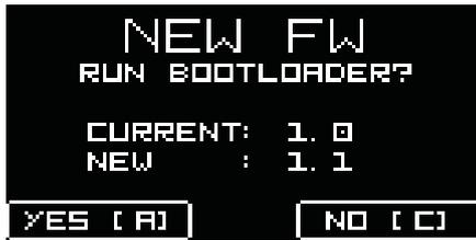
Power off the Sample Drum. Copy the latest firmware file to the root directory of the SD card and insert the SD card in the module and power it on. The module will automatically detect the latest firmware version on the SD card and compare it with the one installed.
