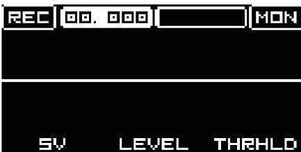
In order to ensure the good quality of recorded samples, before recording you may want to adjust RANGE and LEVEL using encoders D/BACK, E respectively.
