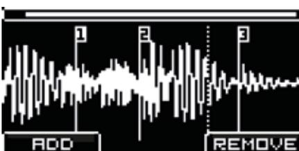
Rotate the encoder E to move slicing cursor left or right and push the encoder A/DATA (ADD) to add the slice point! Maximum number of slices per sample is 32. Slice points will be automatically numbered sequentially.
