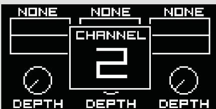
To assign the second channel (bottom row CV1, CV2, CV3) flip the switch to the channel 2 and repeat assign operations, described above.
