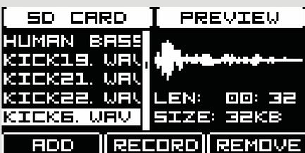
Push the TRG1/PLAY button to listen to the sample! You can preview samples on both SD card and RAM side – the module will preview the last selected sample – use A/DATA and C encoders to navigate through the list of samples. Push TRG2/SHIFT to preview the sample waveform, size and length!
