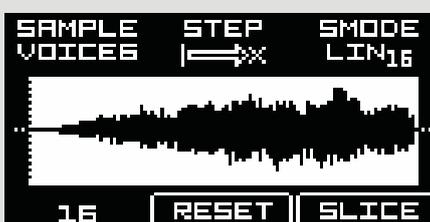
Rotate the encoder C to select slicing mode (SMODE). Available modes for automatic slicing are:
