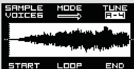
Rotate the encoder C to change the tune of the playback. The Sample Drum supports 1V/oct tuning, and the initial tune is relative – noted by A4. This means – it will play back the sample in the tune as it was originally recorded. It does not mean that it's necessarily A4. Hold TRG2/SHIFT to change the tune by cents. A + or - symbol will appear next to the note for a sample which is also tuned by cents not just semitones.
