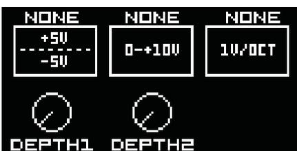
You can also adjust the CV input range by holding SHIFT and rotating the encoders A, B and C.
