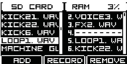
Use the C encoder to navigate through the samples in the RAM. You can REMOVE the samples by pushing the C encoder. You can only load the new sample in the empty slot, so use the C encoder to navigate to the empty slot (at the end of the list or in the middle of the list, if the sample in the list was deleted) and push the A/DATA encoder to upload the new sample. Push and hold the C encoder to clear all samples from the RAM in the corresponding side (1 or 2)!
