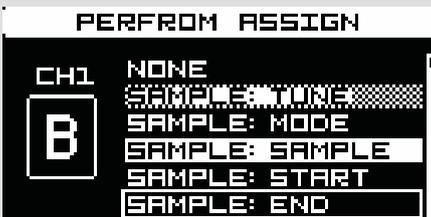
Now use the encoder A/DATA to navigate to the next encoder (B in the example on the left) and rotate the encoder C to assign a parameter to the encoder B, and so on. Parameters assigned to other encoders of the relevant channel (1 or 2) are not available.
