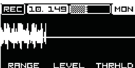
Once RANGE, LEVEL, and THRESHOLD settings are done, push the encoder A/DATA (REC) to start recording. Record timer will indicate the sampling time and level bar will give visual feedback on audio input level.
