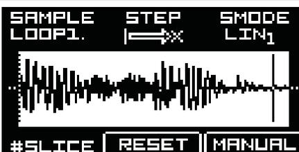
When in sample slicing menu, push and hold TRG2/SHIFT button and push the encoder F to enter the manual slicing mode. Manual slicing screen will appear.
