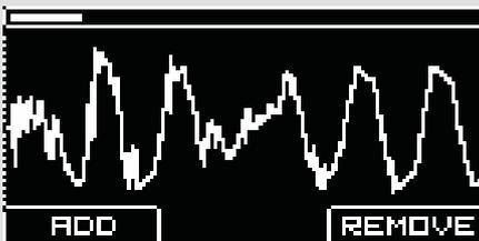
Rotate the encoder C to zoom the waveform! The zoom bar on the top of the screen will show the zoom rate.
