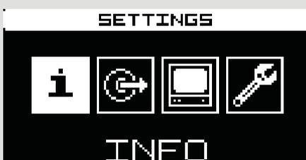
Here you can adjust master settings of the module. Three setting pages are available: System information, Audio output and Display settings. Rotate the encoder A/DATA to navigate to the relevant menu and push to confirm.
