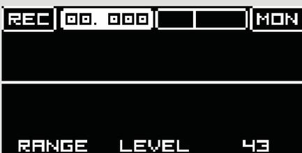
Use the encoder F to set the THRESHOLD of start of the sample record. Meaning, you can set the automatic start of sample record when level of the incoming audio signal reaches certain threshold, for example the first beat of the kick drum.
