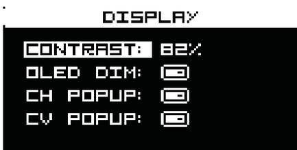
In the Display settings menu you can set the display contrast. OLED auto dimming - this will reduce the contrast automatically if module is not used for 1 minute. Channel popup - with this setting you can enable or disable channel selection popup. CV popup - this option if enabled will show the CV offset for settings which have the CV control enabled.
