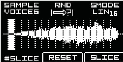
Rotate the encoder B to select slice playback mode, meaning, in what order the slices will be played back with incoming triggers.
