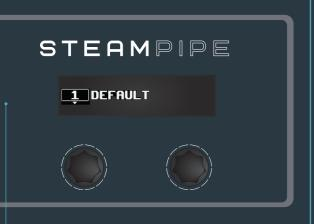
The two encoders are for main menu controls and the OLED display provides visual feedback for the various settings.
