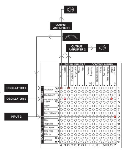
This is an example of a basic patch with EFFECTS. The pulse wave signal from the Oscillator 1 is connected to the input of the VCA (Envelope Signal), and the output of the VCA is routed both to Channel 1 Output and Effects module input. The output of the Effects also is patched to Channel 1 Output. The relation between Envelope Signal level (DRY) and Effects level (WET) settings will provide you desired DRY/WET mix.
