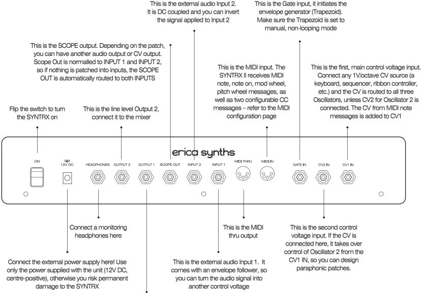
This is the line level Output 1, connect it to the mixer. Depending on the patch, you can achieve nice stereo panning
