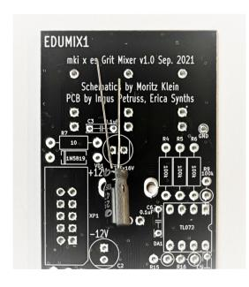
Next, insert & solder the film- and electrolytic capacitors. Electrolytic capacitors are bipolar, and you need to mind their orientation. The positive lead of each electrolytic capacitor is longer, and there's a minus stripe on the side of the capacitor's body to indicate the negative lead. On our PCBs, the positive pad for a capacitor has a square shape, and the negative lead should go into the pad next to the notch on the silkscreen.
