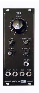
Install the front panel and fix it in place with the 5 hex nuts on the jack sockets and a washer plus hex nut on the top potentiometer. Fit the large knob on the bare potentiometer shaft and fix it in place with a small screwdriver. We are almost done
