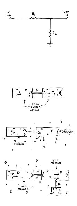
A voltage divider is really just two resistors set up like this: input on the left, output on the right. If R1 and R2 are of the same value, the output voltage will be half of what the input voltage is. How does it work?
