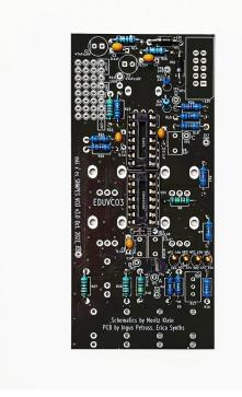
Next up: inserting & soldering the NTC thermistors and transistors. Make sure you place the transistors in their designated spots. Also, they need to be properly aligned with the marked outline on the silkscreen – orientation is critically important here.
