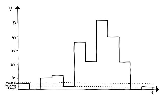
Here's a sequence I drew up as an example. It spans 5 octaves, with the lowest note being a low C at 0 V and the highest a C4 at 5 V. To contrast this, I've marked our transistor's usable voltage range. **As you can see, our sequence is near completely outside of those bounds**. There are two major problems. First, the sequence is just "too big". And second, it's centered way too low – because our transistor is completely shut off at 0 V base voltage.
