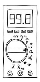
Multimeters come in different shapes and sizes, but the most common type is probably the hand-held, battery powered variant. These can measure a bunch of different things: voltage, current, resistance, continuity. Some have additional capabilities, allowing you to check capacitance, oscillation frequency or the forward voltage drop of a diode.
