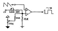
Now while you could exactly calculate the needed resistor values for those parameters, I chose to go with trial & error. And the value that worked best for me was a 68k resistor for the external CV. Also, I decided to add a 250k potentiometer in series here, so you can adjust the CV intensity on the fly.
