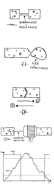
We'll tackle resistors first. While a conductive piece of wire is like a very big pipe where lots of water can pass through, a resistor is like a narrow pipe that restricts the amount of water that can flow. The narrowness of that pipe is equivalent to the resistance value, measured in ohms. The higher that value, the tighter the pipe.
