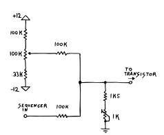
And this is what our completed scaling and offset circuit looks like. Note how I've chosen to combine a fixed 1k5 resistor with 1k precision trimmer. When you set up resistors like this, their values are simply added together. Since the correct value is going to be somewhere between 1k5 and 2k5, this gives us even finer control. Which will make the tuning process a lot less tedious.
