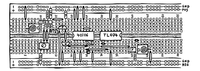
Now in order to tune your VCO properly, you'll need something like a sequencer or a CV keyboard. Here's how it works. I like to dial four steps on my sequencer to a low C (0 V), four more steps to a high C (5 V) and then let it run that sequence in a loop.<sup>16</sup> To make your life a little easier, you should use some sort of digital tuner. You could of course do this by ear, but I've found that that's really rather difficult.
