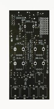
Now, turn the PCB around and inspect your solder joints. **Make sure all components are soldered properly and there are no cold solder joints or accidental shorts.** Clean the PCB to remove extra flux, if necessary.
