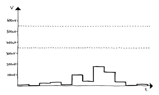
Okay, so our sequence is tiny enough now. But it's still not centered correctly – so we need to shift its center upwards quite a bit. For that, we can do the reverse of something we did before. Remember what an offset voltage is? It's basically a constant voltage that a changing voltage is riding on top of. This is exactly what we need here, so instead of removing it like last time, we'll be adding it our sequence.
