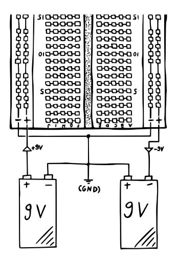
By connecting the batteries like this, the row on the left side labeled + becomes your positive rail, the row on the right side labeled + becomes your negative rail, and both rows labeled – become your ground rails.<sup>4</sup> Please make sure you disconnect the batteries from your breadboard when you make changes to the circuit! Otherwise you run the risk of damaging components.
