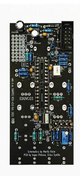
Next, solder the precision trimmer and the power supply socket. Make sure the Insert the jack sockets and solder them.orientation of the socket is as shown in the picture below – the arrow pointing to the first pin is aligned with a notch on the silkscreen. The key on the socket will be facing outwards from the PCB.
