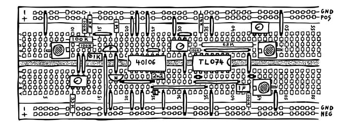
If you have an LFO (low frequency oscillator), you can now try and connect it to the circuit. You should then be able to see something happening on the oscilloscope. If you turn the CV intensity up, you can test if it is indeed going through zero. (If that's what you want!)
