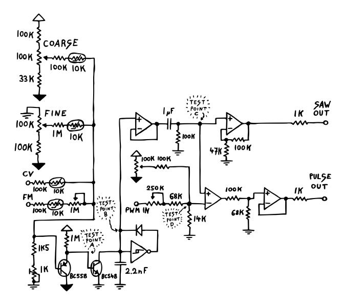
Here's what I came up with: an analog sawtooth-core oscillator with reasonably accurate volt/octave tracking, made from just a handful of basic components.
