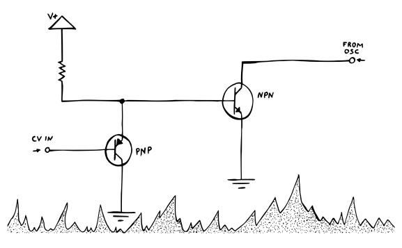
Let's assume we connect the emitter follower to our current sinking NPN transistor like this. That means that any voltage level at the PNP's base would be copied to its emitter and thereby applied to the NPN's base. So actually – it looks like we haven't accomplished anything? That would be true if we ignored the whole deal with transistors and temperature.
