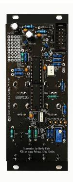
Now, **insert the ICs into their respective DIP sockets.** Mind the orientation of the ICs – match the notch on each IC with the one on its socket.
