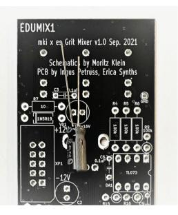
Next, insert & solder the film- and electrolytic capacitors. Electrolytic capacitors are bipolar, and you need to mind their orientation. The positive lead of each electrolytic capacitor is longer, and there's a minus stripe on the side of the capacitor's body to indicate the negative lead. On our PCBs, the positive pad for a capacitor has a square shape, and the negative lead should go into the pad next to the notch on the silkscreen.
