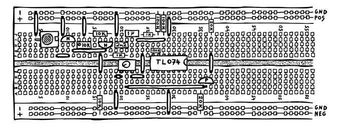
Once you've set this up, try fiddling with the potentiometer. You should see the shape of the output signal change as the folding effect gets more intense.
