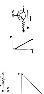
So when the components are paired up, we can see that their behaviors are clashing: while the transistor wants to ramp up its current throughput exponentially, the resistor only allows for a linear increase.
