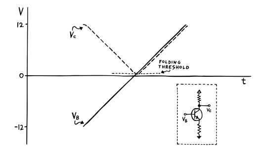
In the region between -12 V and around 450 mV, everything works as expected: the collector voltage (Vc) drops in sync with the base voltage. But after the base- and collector voltages meet, something strange happens: the collector voltage starts rising again. What's up with that?
