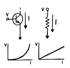
These two components in conjunction serve one simple purpose. **They're meant to convert voltage into current**. More precisely: the voltage we apply to the base into a current flowing through transistor and resistor. Okay, but what is the relation between those two variables?
