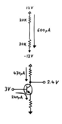
Well, we've run into a phenomenon called transistor saturation. This happens when we try to pull more current into the collector than is available. Think of it like this: If we'd remove the transistor from our circuit, we'd see 600  $\mu$ A flow through both resistors. And we can't increase that current without bumping the voltage or reducing the resistance.
