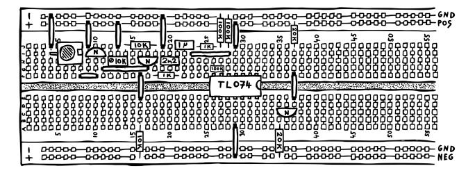
To check on your triangle, connect your oscilloscope to the op amp's output.
