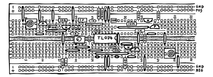
Once you've set this up, check if the signal does pass through unchanged at minimum intensity. Then, see what happens as you dial it up. You should get additional spikes in the output that make it sound even more harsh and metallic.
