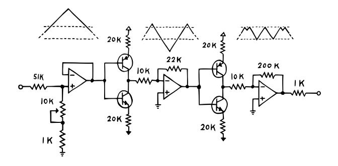
Why is that? Because coming into the second stage, the signal will now wiggle across the thresholds one additional time. In my experiments, increasing the gain by a factor of around 2 gave me the best results. So we'll replace the 10k feedback resistor with a 22k.
