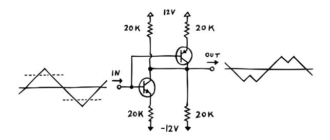
If we then send in our triangle wave on the left, we can pick up a top- and bottom-folded output on the right. It works like this: at 0 V base voltage, without a connection between the collectors, the NPN's collector would sit at +700 mV, while the PNP's collector would sit at -700 mV. Wire them together, and we get 0 V – since the two voltages cancel each other out.
