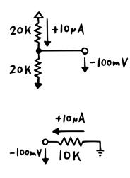
Since this is a 50% voltage divider between +12 V and -12 V, the central node sits at 0 V. At least until we start drawing current from it. Then, the voltage will drop by 100 mV for every additional 10  $\mu$ A we pull through the top resistor.
