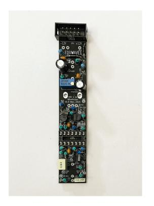
Then insert and solder **the transistors**. Make sure you place correct transistors in relevant places (we use both NPN BC548 and PNP BC558) and align them with the marked outline on the silkscreen – **orientation is critically important here**. Also, insert film capacitors and solder them.
