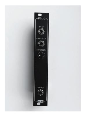
Then fit the **front panel** and fix it with the hex nuts.
