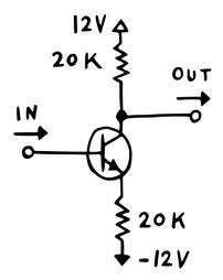
Now, if you've worked with NPN transistors before, you might say "hold on – how is this a wavefolder? It's just a bog-standard amplifier!" And you would be right. What's worse: it doesn't really amplify anything, since it has a gain of -1. So all it does is invert the input signal while keeping the volume the same.
