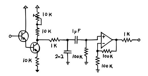
Note that the buffer transistor will add a bit of a negative offset to the input sawtooth – so once you've set this up, you'll have to fiddle with the trimmer again to get the best results. For the op-amp, we'll be using a TL074 IC, which is four op-amps in a single chip. Make sure that you set it up exactly as shown here – if you reverse the power connections, it will heat up and die!
