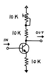
There's a problem with that approach, though. **Every transistor is different from the next when it comes to its "natural" folding threshold (i.e. the one we're getting with equal resistor values)**. The 450 mV we've been assuming so far are just a rough average.
