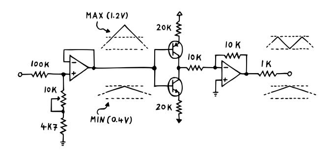
For that, it makes sense to restrict the input volume's range somewhat. If the intensity knob is dialed all the way down, you'd expect the input signal to just pass through the circuit unaffected instead of going completely silent.
