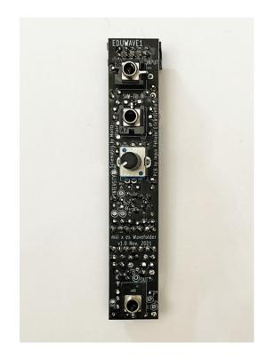
Now, turn the PCB around and inspect your solder joints. **Make sure all** components are soldered properly and there are no cold solder joints or accidental shorts. Clean the PCB to remove extra flux, if necessary.
