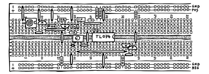
If you again check on the voltage at the two transistors' collectors with your oscilloscope, you should see both the top and bottom of the input triangle get folded over.<sup>16</sup> Perfect! So how do we listen to this now? **Unfortunately, we can't just attach an output socket to the transistors' collectors, since that would mess with the core mechanism by pulling more current through it**.
