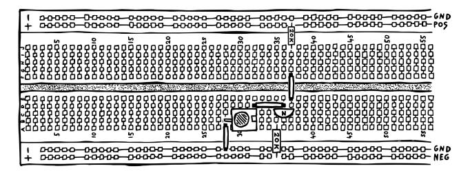
If you now send a triangle, sine or sawtooth wave into the jack socket connected to the transistor's base while monitoring the voltage at the collector with an oscilloscope, you should see some folding happening.<sup>8</sup>
