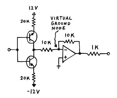
This approach has two benefits. First: we undo the inversion that the wavefolding stage applies to the input signal. So the output will be in phase with the input again. And second, the new 10k resistor gets to work double duty: it's providing the extra current for our two transistors – and it's playing its role as input resistor for the inverting buffer.
