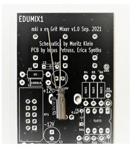
Next up: insert & solder the electrolytic capacitors. Electrolytic capacitors are bipolar, and you need to mind their orientation. The positive lead of each electrolytic capacitor is longer, and there is a minus stripe on the side of the capacitor's body to indicate the negative lead. On our PCBs, the positive pad for the capacitor has a square shape, and the negative lead should go into the pad next to the notch on the silkscreen.
