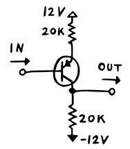
As you can see, the only real difference here is in the type of transistor we're using. I've simply replaced the NPN with a PNP transistor. And since the PNP transistor is basically just the NPN transistor's bizarro twin brother, everything about it is inverted. Collector and emitter switch positions, and the current flowing through them increases as the base voltage decreases.
