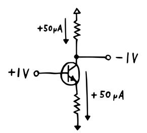
Which, in turn, means that we have to pull that current through the top resistor. And because that resistor is of the same value as the one at the bottom, the voltage below it will drop by exactly 1 V. There are two caveats here, though. First, the absolute collector voltage will be a small but fixed amount higher than the base voltage.
