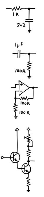
Unfortunately, there's not much we can do to prevent this from happening. So instead, we'll rely on a simple, but effective fix: **applying a low-pass filter to our sawto-tri converter's output**. This will cause the gap between the triangle's sides to be smoothed, resulting in less noticeable buzz in the output signal. In my experiments, combining a 1k series resistor with a 2.2 nF capacitor to ground gave me decent enough results.
