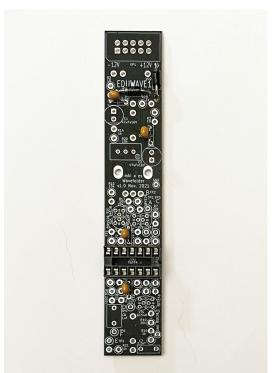
I usually start populating PCBs with lower, horizontally placed components. In this case, these are power protection diodes. Bend the diode leads and insert them in the relevant places according to the part placement diagram above. Remember when inserting the diodes, orientation is critical! A thick white or black stripe on the PCB indicates the cathode of a diode match it with the stripe on the component. Flip the PCB over and solder all components. Then, use pliers to cut off the excess leads.
