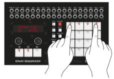
2) Press and hold down the STEP KEY 1 and while holding it down press the STEP KEY 4. Now all STEP keys of the first row will light up – that means that the patterns are linked.
