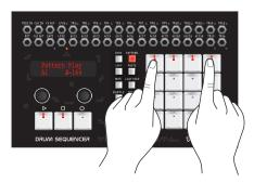
2) Press and hold down the STEP KEY 1 and while holding it down press the STEP KEY 4. Now all STEP keys of the first row will light up - that means that the patterns are linked.3) To unlink patterns and continue to play one pattern press any of the STEP KEYS.
