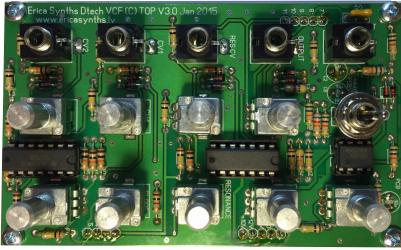
Solder extended connector jacks on the bottom PCB! Use screwdriver to push down top spacer. Then cut connectors 18mm high.
