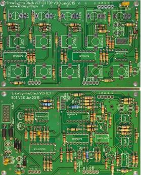
3 Turn the bottom PCB around and solder eurorack power connector and trimpots.
