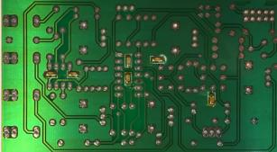
2 Solder all passive elements, diodes and then IC sockets.
