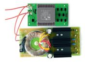
One side of Erica Fusion PSU 6VAC output has to be connected to the GND of your modular system. Use the wire supplied with the kit to do so. Since 6VAC circuit is isolated, if you connect this wire somewhere incorrectly. But that may affect quality of sound of Erica Fusion models.
