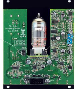
For +-12V operation install 2 jumpers on the Fusion PSU connector as shown on the picture. If you use this module with the Erica Fusion PSU, no need to install these jumpers. You connect Fusion PSU ribbon cable here.
