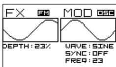
Let's explore the **FM EFFECT!** Push the left encoder to access the DEPTH setting - relative maximum value (depth) for which the frequency modulation will be performed, in other words - the depth of the frequency modulation when FX
