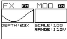
**IF THE EXTERNAL MODULATOR IS SELECTED (IN)**, you can apply the modulation CV (LFO, envelope generator or any other modulation source) to the FX CV input, and adjust its amplitude with the FX CV potentiometer.
