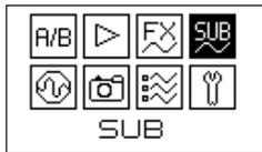
In Suboscillator configuration menu you can alter suboscillator settings. The suboscillator is assigned to the OUT2. No FX (except frequency modulation) is applied on the suboscillator.
