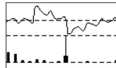
The wave with the corresponding spectrum of harmonics will appear on the screen. You also can alter the wave by adjusting harmonics. Use the left encoder to navigate thru harmonics (selected one gets bolder) and the right one to adjust amplitude of the harmonic.
