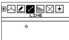
In **LINE SKETCH** mode you can draw the wave by connecting lines between two points defined by cursor. move the cursor to desired position and push the left encoder to initiate drawing.
