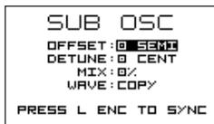
Rotate the left encoder to select settings you wish to alter and rotate the right one to alter the setting. Click the encoder to confirm.
