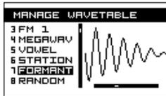
As the bank is selected, you can use MORPH knob to browse through the waves in the bank and hear, how the bank sounds. You can design wavetables in Wave list menu or in the Graphic VCO Google App (see below). Waves added to the wavetables are automatically morphed for the best sound.
