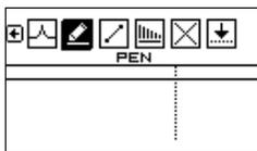
In the **PEN SKETCH** mode you just use both encoders to draw the wave form scratch. The left encoder moves drawing cursor up and down, the right - right. Push the right encoder to initiate drawing. The cursor will change to small cross.
