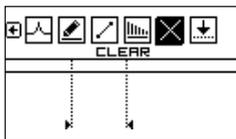
To **DRAW A NEW WAVEFORM**, load any waveform, select edit mode, delete the wave and start design from scratch. Or select NEW in the MANAGE menu.
