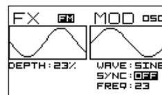
With SYNC: OFF you can adjust the internal oscillator frequency. Rotate the FX potentiometer to set the frequency from 0.13Hz to 4000Hz.
