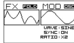
**FOLD AND WRAP FX** provides you distinct wavefolder or wavewrapper. Rotate the right encoder to select between wavefolder (FOLD) or wavewrapper (WRAP). Push the right encoder to access GAIN adjustment and OFFSET adjustment if you use an
