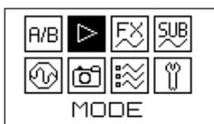
Let's start with **SELECTING OPERATING** (playback) **MODE!** Use the left encoder to navigate thru screen and push the encoder to confirm the selection.
