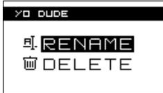
To delete or rename the snapshot, push and hold the left encoder for 1" and delete/rename screen will appear.
