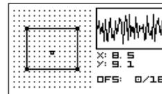
You can alter the size of the matrix by clicking the left encoder. At the first click the bold dot in the top left corner will appear and you can adjust the size of the matrix by rotating left and right encoders, at the second click the bold dot will appear in the bottom
