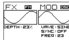
Let's start with the **INTERNAL MODULATION OSCILLATOR (OSC)**. First, you have selection of the waveforms (WAVE). Rotate the right encoder to browse the waveforms. Available waveforms are: Sine, Triangle, Ramp, Sawtooth, Square, Sample&Hold. Note that not all modulation waveforms will give nice resulting sound. We recommend to begin experiments with the sinewave.
