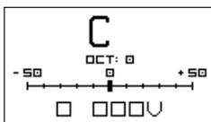
The oscilloscope configuration menu you can use the left encoder to browse thru menu shows current tune of the VCO in semitones and cents,  $\nu$ /oct input status, and rotate it to adjust settings.
