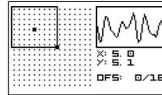
X and Y under the oscilloscope screen represent currently selected wave position, while OFS - allows you to offset all wavetables in the screen up. For example, if you have 32 wavetables in total then OFS: 2/16 will mean that the screen indicates wavetables from 3 to 18. You can change the offset position by clicking and rotating the right encoder.
