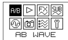
The **BASIC MODE** is **WAVE DESIGN** and Morphing between waves A and B. In this mode you can use encoders to draw two waves - A and B (or select ones from the list) and morph between them manually or via Morph CV, thus getting interesting in-between waveforms. Futuremore, you can alter
