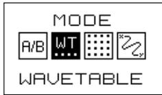
In Wavetable menu you can select wavetables of 16 waves from the list of BANKS and play them back, while morphing thru waves using MORPH knob or Morph CV.
