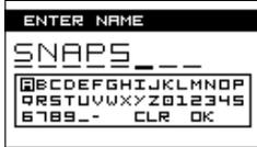
As the snapshot is saved, the snapshot name menu will appear. Use the right encoder to navigate thru characters and click to confirm the selection. Click OK to confirm the name.
