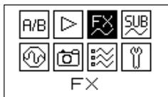
In FX menu you can apply several effects on the waves being played back. FXes are master settings and they are applied on the resulting wave before the output. FXes (except frequency modulation) are NOT applied to the suboscillator.
