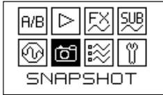
Once you are happy how your designed waves or wavetables with suboscillator configuration and FXes applied sound you can save a SNAPSHOT – a combination of all your settings for a specific sound, which can be instantly recalled during the performance.
