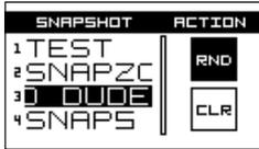
To recall the snapshot, open the snapshots menu and use the left encoder to select the snapshot from the list. Click the encoder to confirm the selection.
