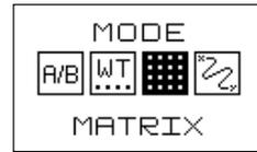
In Wavetable Matrix mode you have your wavetables and waves displayed as a matrix, where rows represent wavetables (wavetables appear in the order as set in MANAGE menu) and columns - individual waves. All waves are represented as dots in the matrix and active wave - one which is played back - as bolder dot.
