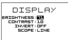
In the display configuration menu you can adjust display brightness, contrast and invert the display appearance to the black background. Use the left encoder to browse thru menu and rotate it to adjust settings. If you wish to film a demo of the module, we recommend to set minimum brightness ;)
