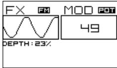
For some effects (specifically, phase distortion, wavefold, wave wrap, bitcrush) **MANUAL CONTROL (POT)** over the effect gives nice results. Just use the FX potentiometer to alter the waveshape.
