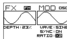
With SYNC: ON you can select synchronization ratio. Rotate the FX potentiometer to desired sync ratio (the module provides both multiplied and divided frequencies). Note that module will play back the resulting wave in real time and you can hear modulation sweetspots.
