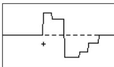
You can't move the cursor left, as the wave should change over the time, and it can't go back in the past. We recommend to draw waves that start and end at horizontal axis otherwise you may hear undesired clicks.
