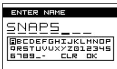
The name screen will appear and you can name the waveform. It will be saved as the last in the waveform list. See the Waveform and wavetable management procedures below.
