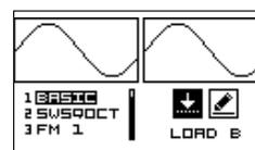
To do so, click the left encoder on the **LOAD** icon to load the waveforms in the left window and click the right encoder to load waveforms in the right window.
