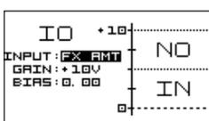
In the IN/OUT configuration menu you can configure CV inputs by adjusting their gain, and bias. Use the left encoder to select the input or setting and right one to adjust the amount of the setting.
