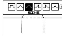
Once you have clear screen, you can draw one period of the wave and simultaneously listen to the result. To do so, use the left encoder to select the principal waveform, you wish to start with, from the icons above and click to confirm selection. Available principal waveforms are pulse, triangle, sine, ramp, sawtooth and logarithmic sine. Example shows sine waveform selected.
