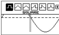
In the wave edit mode you'll see the waveform and by **PUSHING THE LEFT** encoder, you'll access the wave edit menu on the top of the screen. Rotate the left encoder to access wave edit options! **Editing waveforms is similar to designing the new one - please,**
