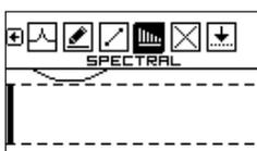
As you draw the wave, you can check the **HARMONIC CONTENT** of it, specifically, the first 32 harmonics. To do so, use the left encoder to select SPECTRAL icon in the top row.
