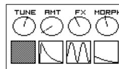
Push the left encoder to access controls status menu – it shows the position of controls and inputs used for the specific snapshot. In example on the left you can see the settings of the potentiometers and CV shapes applied to CV inputs.
