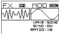
**RINGMODULATOR** works similar to the FM. The principal oscillator is considered a main signal, but Modulation oscillator or signal applied to the FX CV – a carrier.
