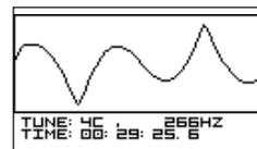
It also indicates the tune of the VCO in notes and Hz, as well as time passed from the powering on the modular system. If you wish to reset the timer to keep timing of your performance, just push the right encoder and the timer will reset to 0.
