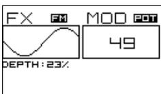
On the right side of the screen you have modulator settings. There are three options: POT (potentiometer), external modulation input (IN) and the internal modulation oscillator (OSC). Rotate the right encoder to select one of those! Push the encoder to access the next modulator setting!
