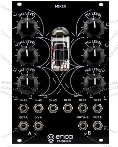
Input attenuators adjust right mixer signal levels. Input accepts signals at virtually any level, because they are fed directly into tube.
