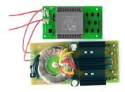
One side of Erica Fusion PSU 6VAC output has to be connected to the GND of your modular system. Use the wire supplied with the kit to do so. Since 6VAC circuit is isolated, nothing wrong or critical will happen, if you connect this wire somewhere incorrectly. But that may affect quality of sound of Erica Fusion modules.
