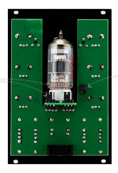
For +-12V operation install 2 jumpers on the Fusion PSU connector as shown on the picture. If you use Fusion Mixer with the Erica Fusion PSU, no need to install these jumpers. You connect Fusion PSU ribbon cable here.
