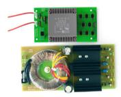
Use wires supplied with the Erica Fusion PSU kit to connect eurorack PSU to relevant lugs on the Fusion PSU module!
