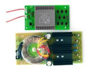
Use wires supplied with the Erica Fusion PSU kit to connect eurorack PSU to relevant lugs on the Fusion PSU module!
