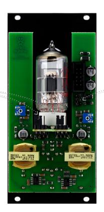
For +-12V operation install 2 jumpers on the Fusion PSU connector as shown on the picture. If you use Fusion Mixer with the Erica Fusion PSU, no need to install these jumpers. You connect Fusion PSU ribbon cable here.
