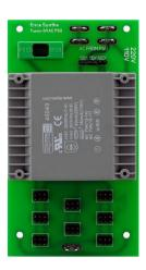
Use spacers and screws supplied with the Erica Fusion PSU kit to fix it in your modular case next to the eurorack power supply unit!
