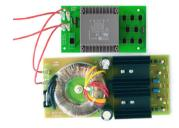
One side of Erica Fusion PSU 6VAC output has to be connected to the GND of your modular system. Use the wire supplied with the kit to do so. Since 6VAC circuit is isolated, nothing wrong or critical will happen, if you connect this wire somewhere incorrectly. But that may affect quality of sound of Erica Fusion modules.
