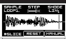
When in sample slicing menu, push and hold TRG2/SHIFT button and push the encoder F to enter the manual slicing mode. Manual slicing screen will appear.
