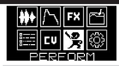
Use the encoder A/DATA to navigate to the PERFORM menu and push to confirm.
