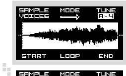
Rotate the encoder C to change the tune of the playback. The Sample Drum supports 1V/oct tuning, and the initial tune is relative – noted by A4. This means – it will play back the sample in the tune as it was originally recorded. It does not mean that it's necessarily A4.
