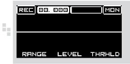
In RECORD mode you can record samples directly to the RAM of the module and afterwards save them to the SD card. Samples are saved as 16bit 48Khz wav files. 12bits is the resolution of the ADC. Maximum record time is 30". To record the sample, patch the audio signal to CV3/REC (bottom row CV3) input.
