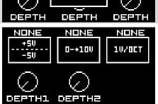
0 to +10V - voltage range usually outputted from envelope generators 1V/Oct - voltage range used by most sequencers (no depth setting on this one)
