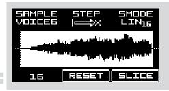
Rotate the encoder C to select slicing mode (SMODE). Available modes for automatic slicing are:
