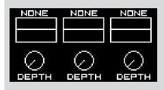
In the CV menu you can assign each of three CV inputs to different parameters of the Sample Drum, like tune, play mode, sample select, start, loop and end point, envelope attack, hold and decay, etc., as well as adjust modulation depth via attenuators.
