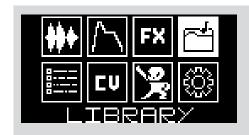
Rotate the A/DATA encoder to navigate to the LIBRARY menu. Click the encoder A/DATA to access the list of the samples on the microSD card!
