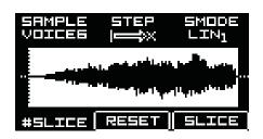
In order to activate sample slicing push the A/DATA encoder. Slicing screen will appear and the encoders will change their functions. To exit slicing mode push the A/DATA encoder again. Rotate the encoder A/DATA to select samples from the RAM. Note that slices are saved on the RAM with the samples and will be saved within the project not the samples on SD card.
