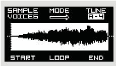
Rotate the encoder C to change the tune of the playback. The Sample Drum supports 1V/oct tuning, and the initial tune is relative – noted by A4. This means – it will play back the sample in the tune as it was originally recorded. It does not mean that it's necessarily A4.
