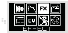
Use the encoder A/DATA to navigate to EFFECT menu and push to confirm.
