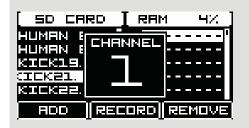
Note that you need to upload samples to both channels 1/2 individually – use the switch to select the channel and upload samples; popup screen will inform you, which channel is currently active. The message in the top right column will indicate RAM usage. Take note that both sides share the same RAM!
