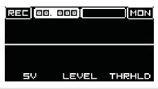
In order to ensure the good quality of recorded samples, before recording you may want to adjust RANGE and LEVEL using encoders D/BACK, E respectively.
