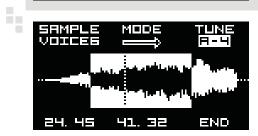
Rotate encoders D/BACK, E and F to select start point, loop point and end point of the sample payback. In loop mode the playback will start at the selected start point, play to the end point and then continue looping between start and loop points. Please note that in loop mode sound can fade out depending on envelope settings. Refer to AMPLITUDE menu on envelope settings.
