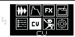
Use the encoder A/DATA to navigate to the CV menu and push to confirm.
