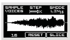
Rotate the encoder C to select slicing mode (SMODE). Available modes for automatic slicing are:
