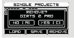
To delete the project, push the encoder C (REMOVE) and confirm YES/NO popup will appear. Rotate the encoder A/DATA to select and push to confirm.
